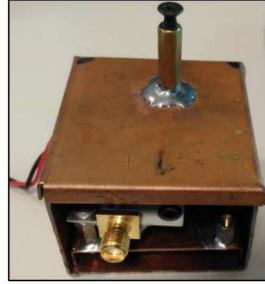
Fig. 4: 18 GHz DRO picture
