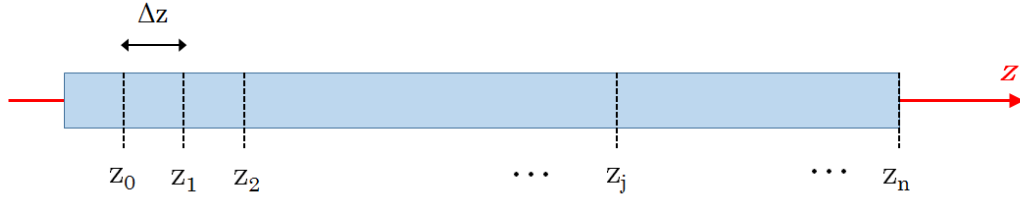
Figure 3.1: Active fiber model showing step size
