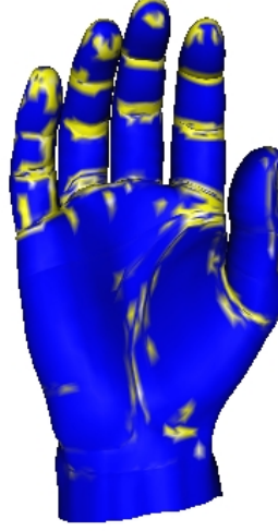
Figure 3.16: Differential velocities on a 3D model. Brighter (yellow) regions express high differential velocities. The figure shows the absolute amounts of differential velocities in a scalar manner for a better presentation.
