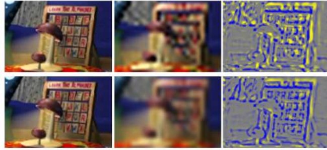
Figure 5.10: Comparison of Upsampling Algorithms. Top-left and Bottom-left: Original image, Top-middle: Level 2 image upsampled with Lanczos filter, Top-right: Intensity contrast change map of top-middle image (compared to the original image), Bottom-middle: Level 2 image upsampled with B-Spline filter, Bottom-right: Intensity contrast change map of bottom-middle image (compared to the original image). (From [20]. ©2010 Elsevier, reprinted with permission.)
