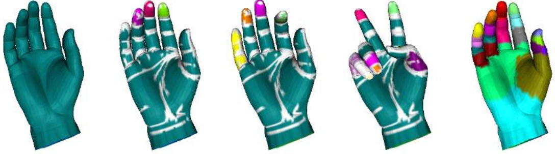
Figure 3.17: Clustering through an animation, from left to right (except the rightmost): clustering results after several frames are shown. White regions depict the boundary vertices. The rightmost image shows the final clustering after clustering refinement phase.
