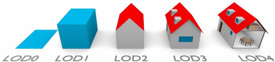
Figure 2.2 Levels of Detail in CityGML by Biljecki et al. [24]
