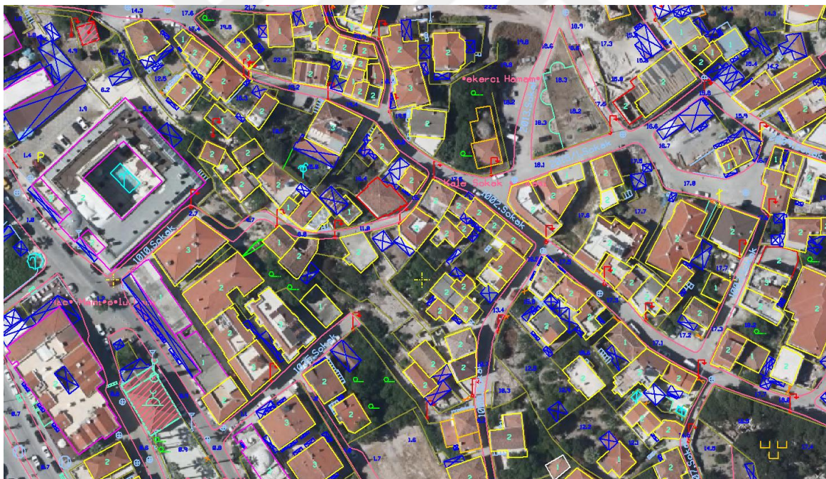
Figure 4.1 Manual feature extraction from stereo aerial images
