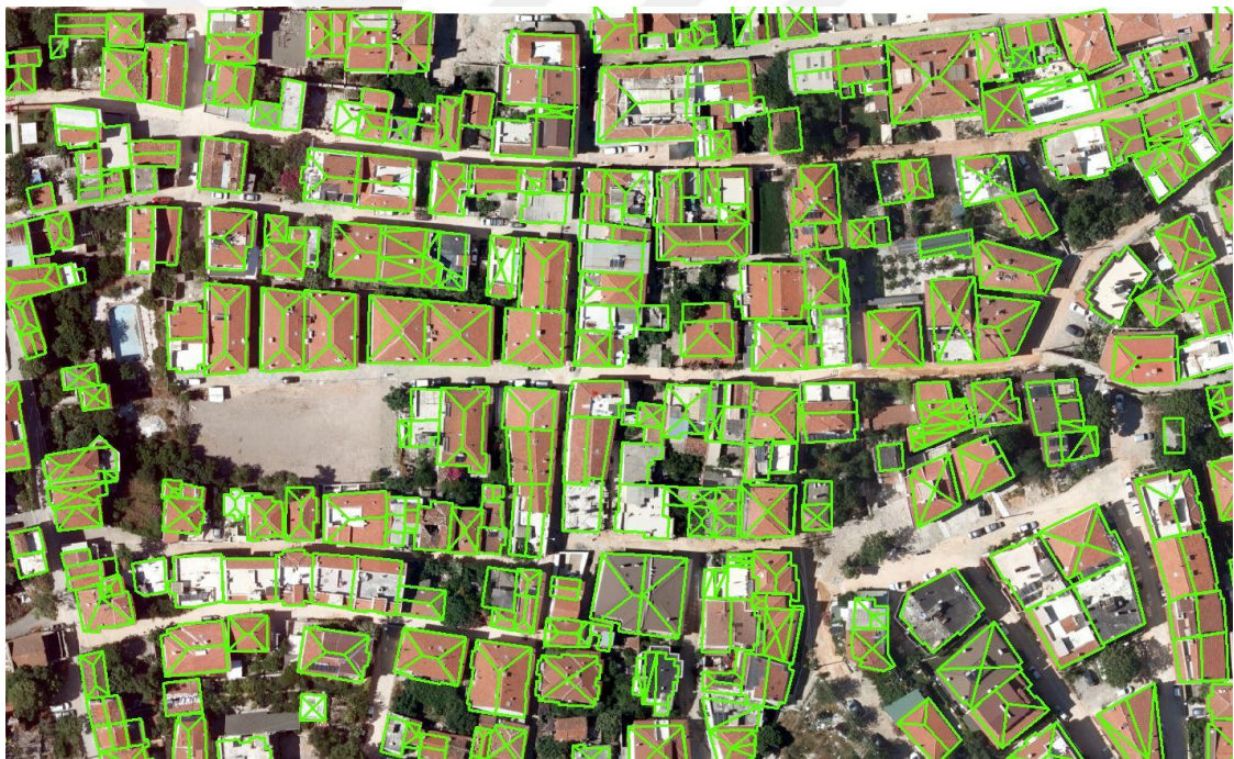
Figure 4.16 Automatically generated roof geometries overlayed on the orthophoto with 10 cm resolution.
