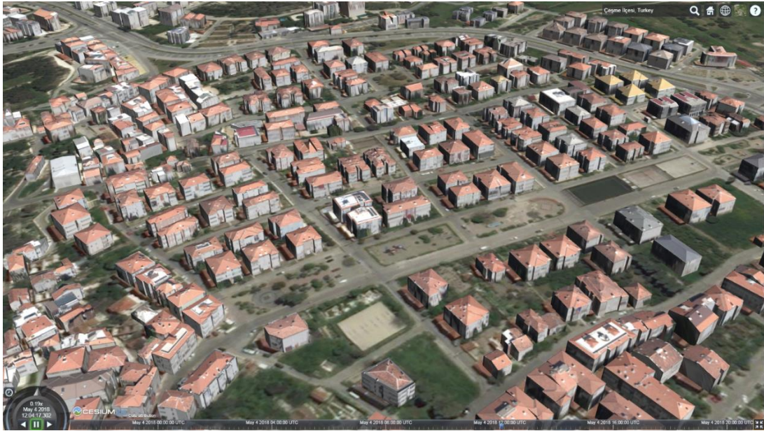
Figure 6.11 Textured CityGML converted to 3D Tiles format and visualized on CesiumJS
