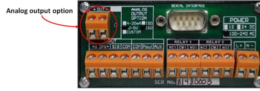
Figure 3.3: Analog option of the Tachometer
