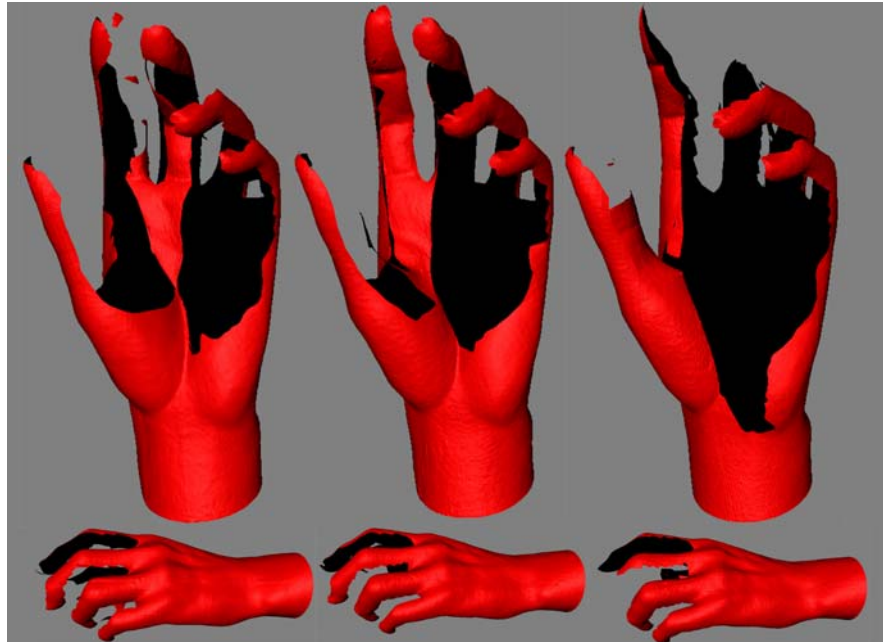
Figure 4.19: Triangulated range surfaces obtained from three separate scans of optical triangulation.
