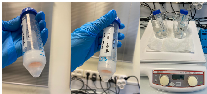
Figure A.3: The assembly utilized for drug release at different pH
