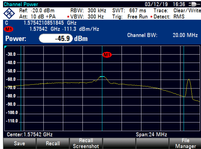
Figure 5.7 Power of the GPS signal after up-conversion at the output of the receiver hardware
