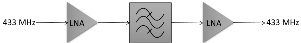
Figure 3.36 Cascaded LNA, BPF, and LNA
