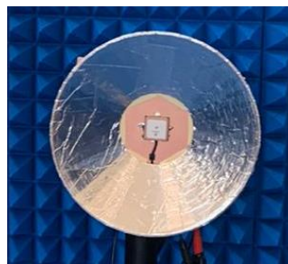
Figure 3.8 Directional outdoor GPS active antenna
