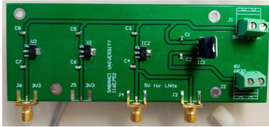
Figure 3.55 Voltage regulator for repeater hardware
