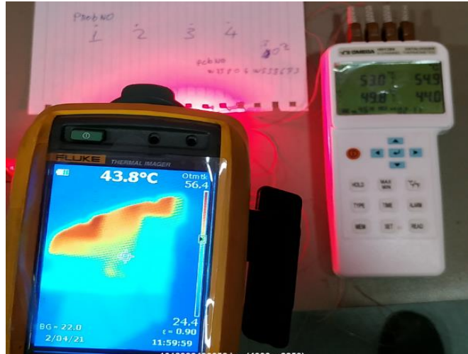
Figure 1.48 Thermal camera and thermocouple calibration.
