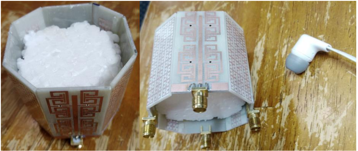
Figure 4.8: Fabricated Prototype of MIMO Antennae Array.
