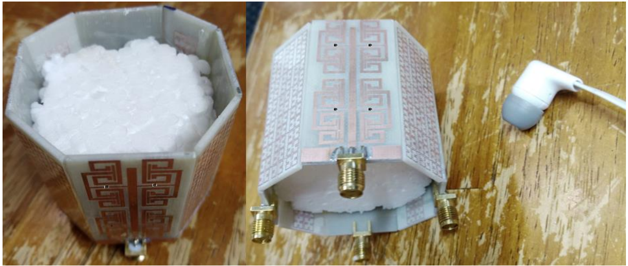
Figure 4.8: Fabricated Prototype of MIMO Antennae Array.
