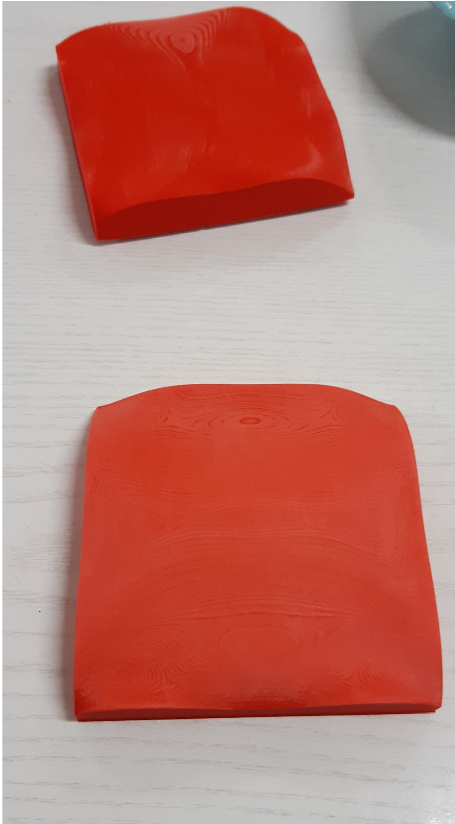
Figure 4.3: Sample printed reflectors before (top) and after (bottom) sanding.
