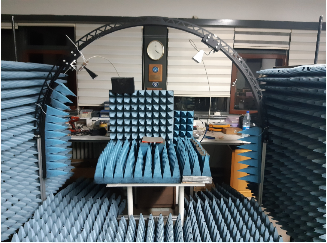
Figure 4.10: A photograph of the NRL arch measurement setup.
