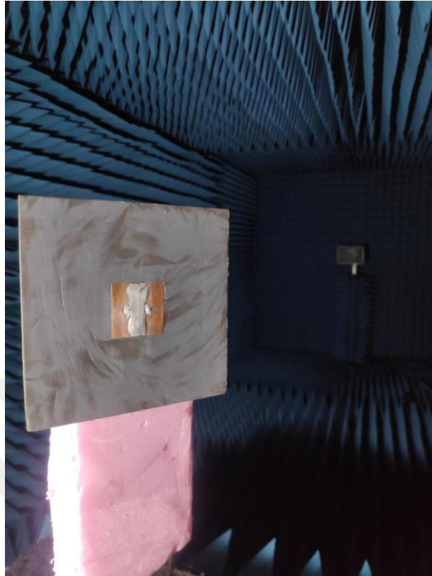
Figure 3.13 Measurement setup of the antenna in the anechoic chamber.
