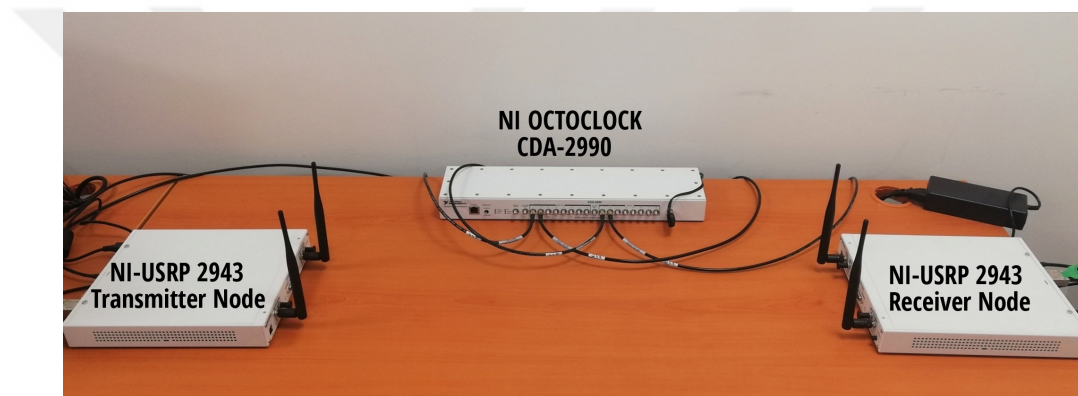
Figure 3.10: Experimental testbed at CoreLab [CoreLab, 2020] with USRP modules.
