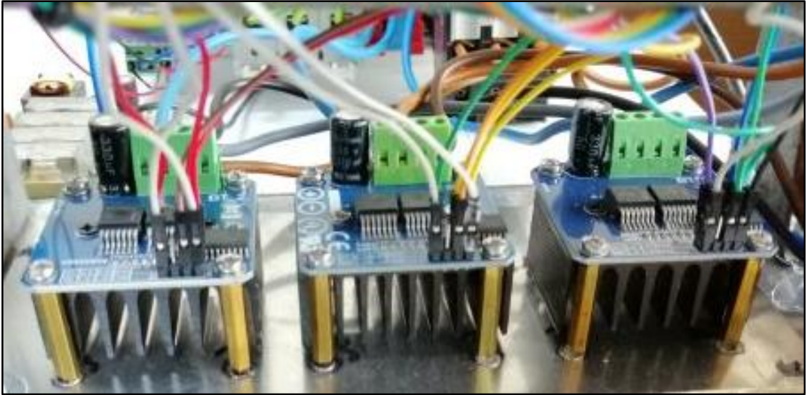
Figure 2.4. Three BTS7960B drivers for three-phase ERSM
