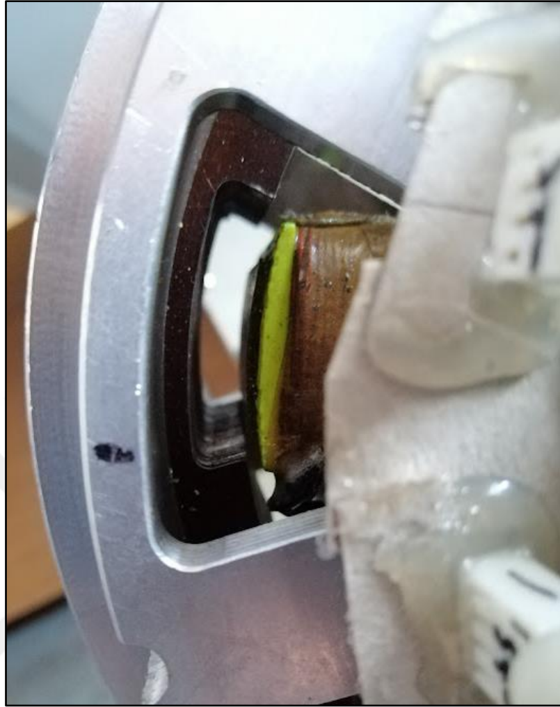
Figure 1.14. The slots on the outer enclosure of the motor prototype.
