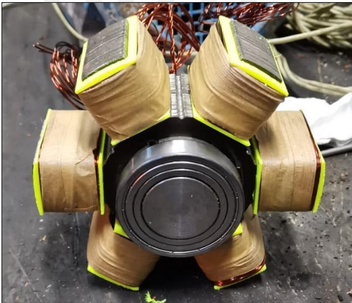
Figure 2.1. SRM stator with coils
