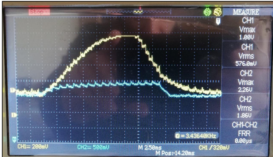
Figure 3.4. Oscilloscope view of the current (blue line) and the flux linkage (yellow line)
