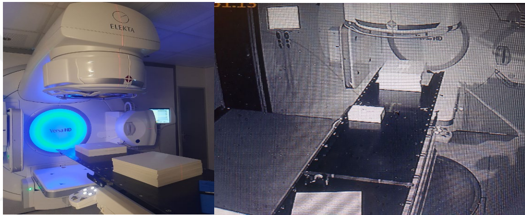
Figure 3.4 Irradiation of gafchromic films
