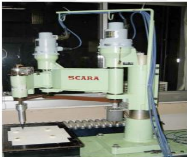
Figure 1.5 One of the first prototypes of Scara robot, designed by Hiroshi M.
