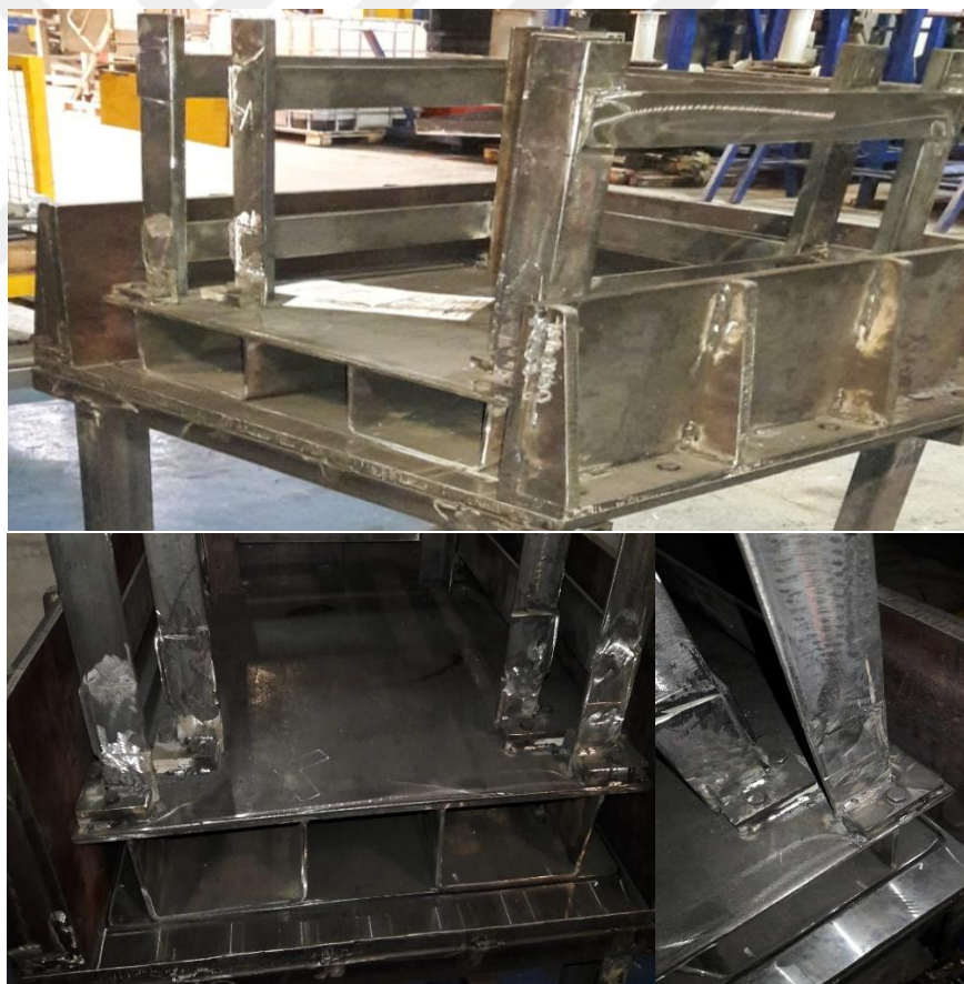
Figure 3.23 View of special purpose stacking carrier
