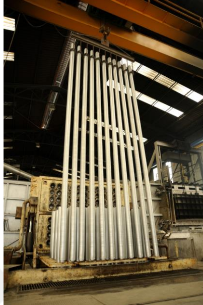
Figure 1.7. Extraction of billets from the casting well (Zahit Aluminium, 2019)
