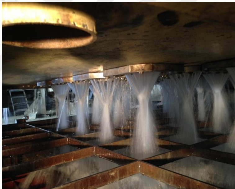
Figure 3.7. Water flow around the molds used on the casting table (Zahit Aluminium, 2019)
