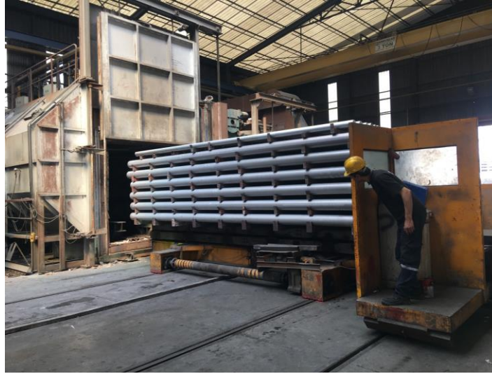
Figure 1.12. Billet loading to the homogenization furnace. (Zahit Aluminium, 2019)
