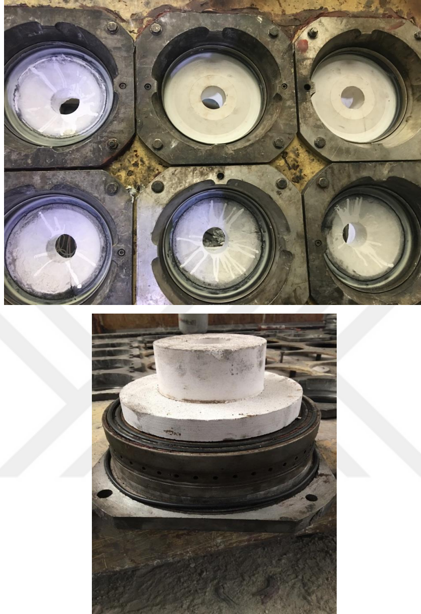
Assembly of 4 thimbles to molds
