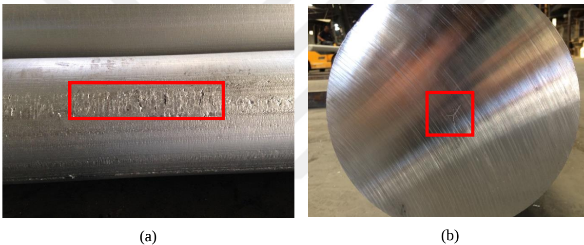
Figure 3.22. Initially, defects on the (a)billet surface and (b)center crack (Zahit Aluminium, 2019)
