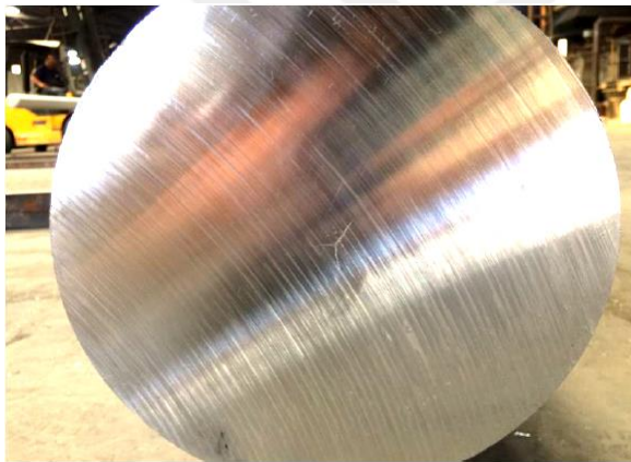
Original casting 203mm initial situation: center crack
