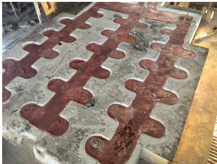
Figure 1.6. Aluminium filled molds (Zahit Aluminium, 2019)
