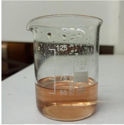
Figure 3.6: Colorization of NaI mixture
