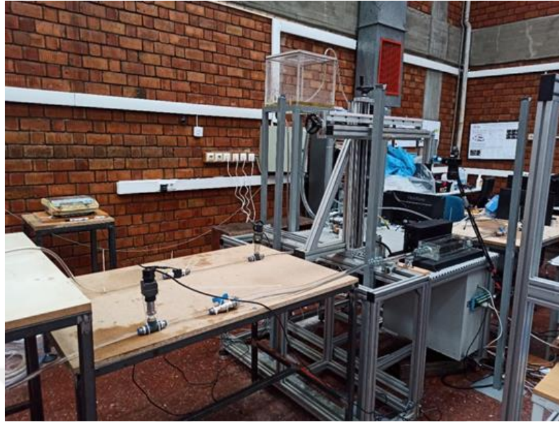
Figure 3.3: Picture of the circulatory system with flowrate and pressure measurement equipment
