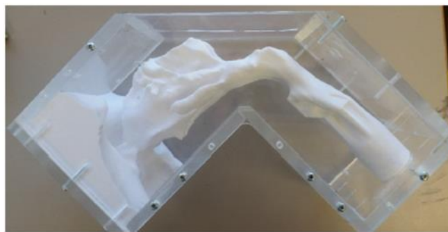
Figure 2.7: Casting box for PDMS with male mold [36]
