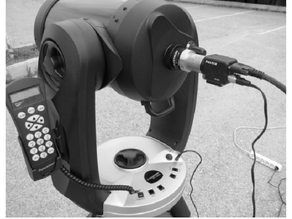
Figure 3.6: The receiver side showing line of sight. and Receiver side connected to CCD camera with an adapter
