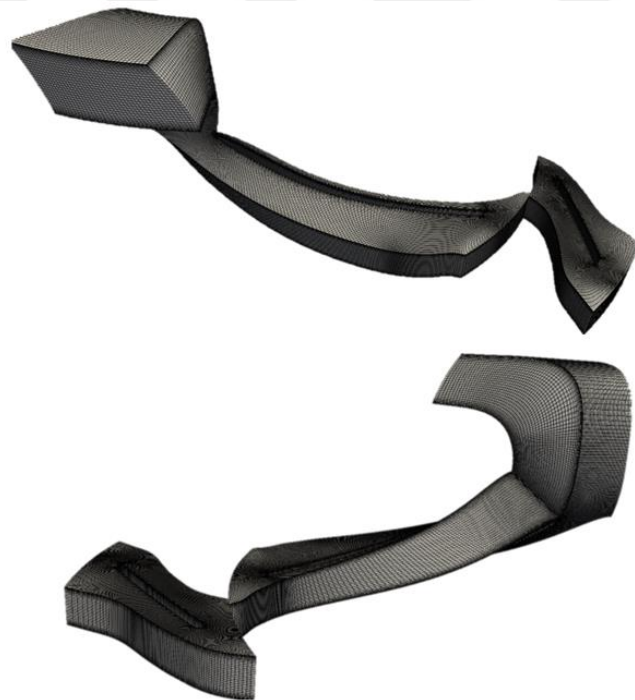
Figure 11: Single passage, multiblock grid for the domain investigated.
