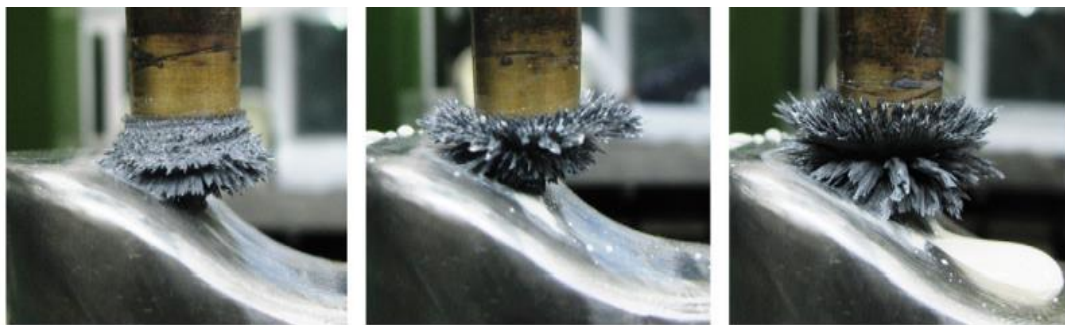
Figure 2.11: Polishing of free-form surfaces with MR fluid brush (Sidpara and Jain, 2013).
