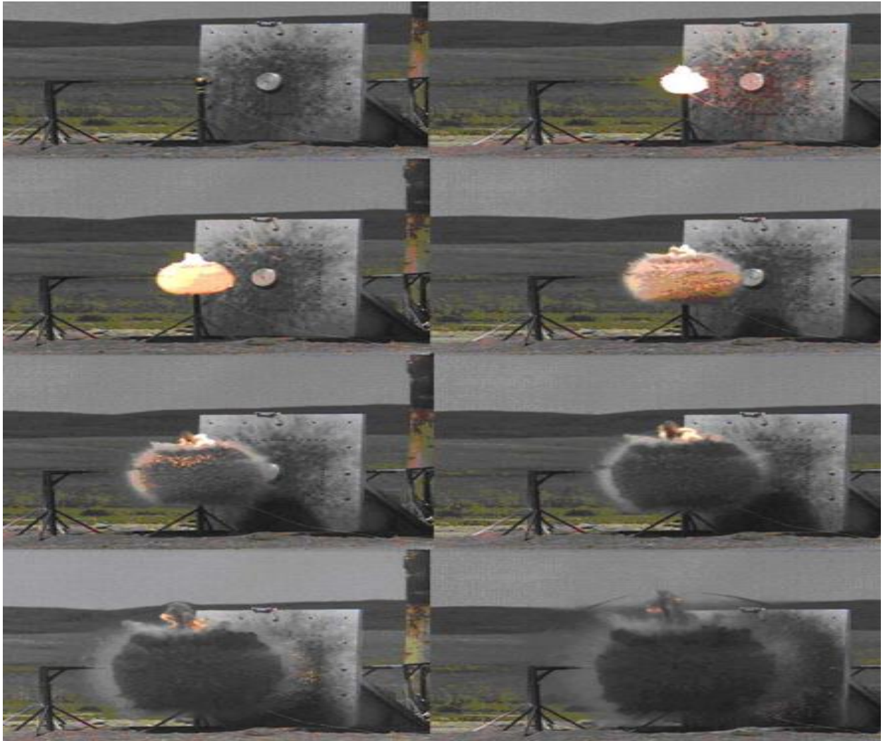
Figure 1.29. High speed photographs of the explosive dispersal of 275 \mu\text{m} steel particles from an 11.8 cm diameter charge. Times are 0, 40, 80, 160, 240, 360, 560 and 840 \mu\text{s} respectively (Frost et al., 2007).
