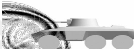
Figure 1.2. Pressure countours of an explosion near an armoured vehicle (Tai et al., 2007)
