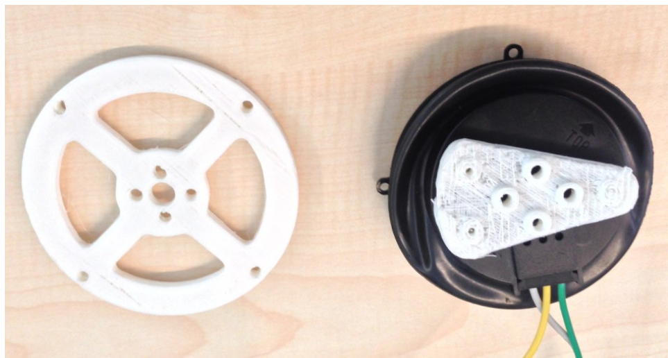
Figure 6.18: Designed adaptor parts are 3D printed as prototypes for corrections.
