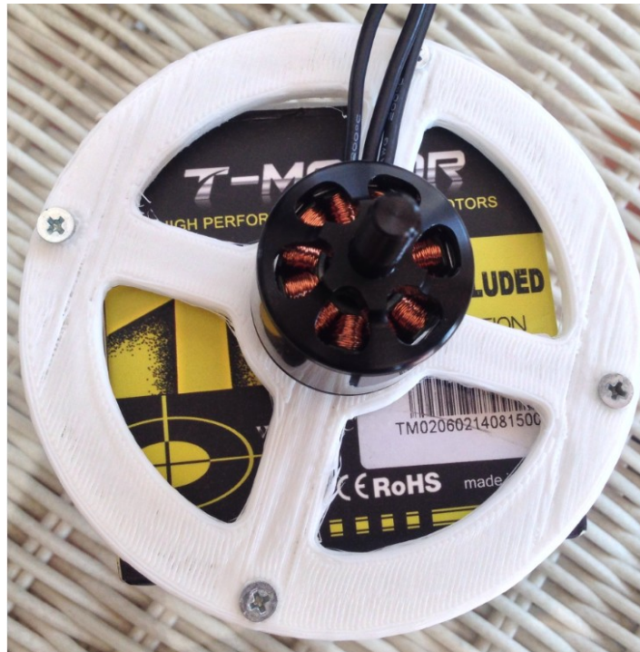
Figure 6.21: Top view of the part 1 assembled with electrical brushless motor.
