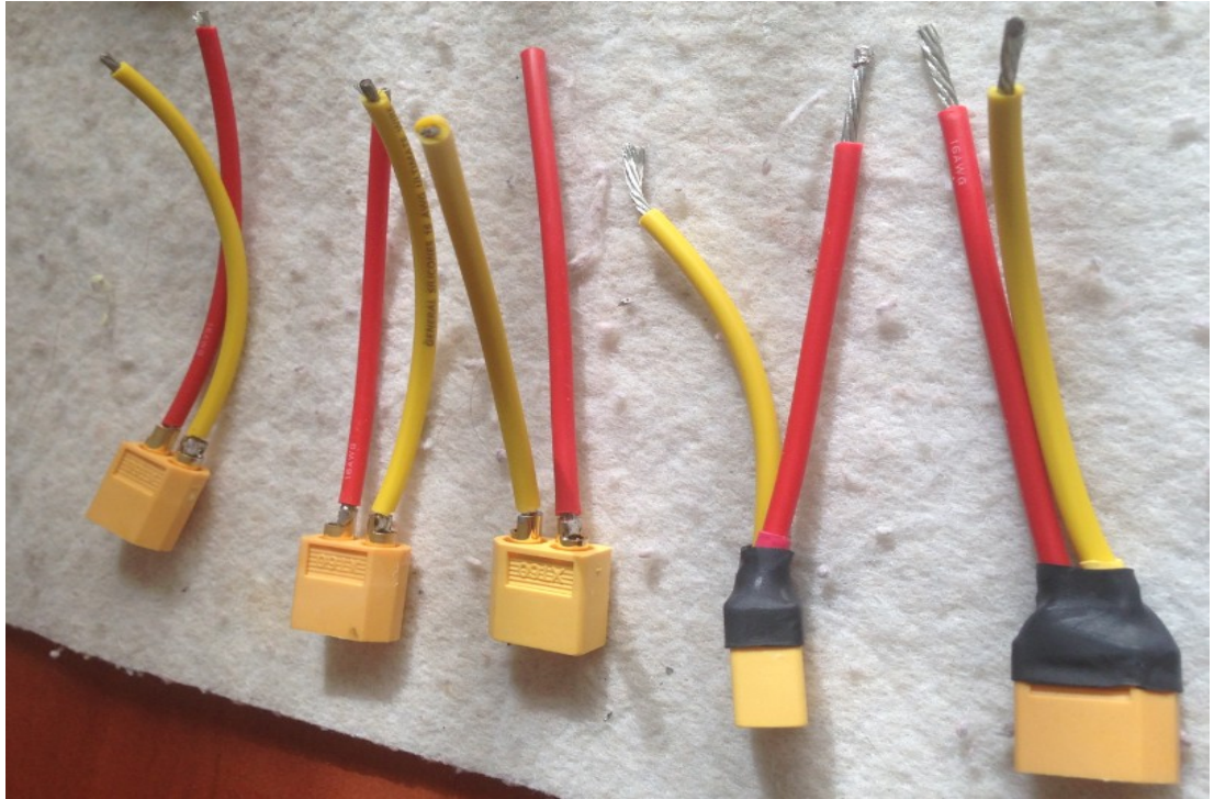
Figure 6.5: Preparation of power cables.
