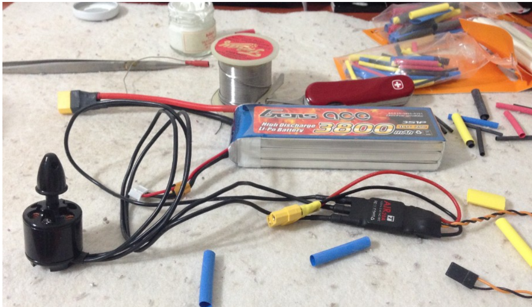
Figure 6.4: ESCs need to be calibrated with intermediate-timing.
