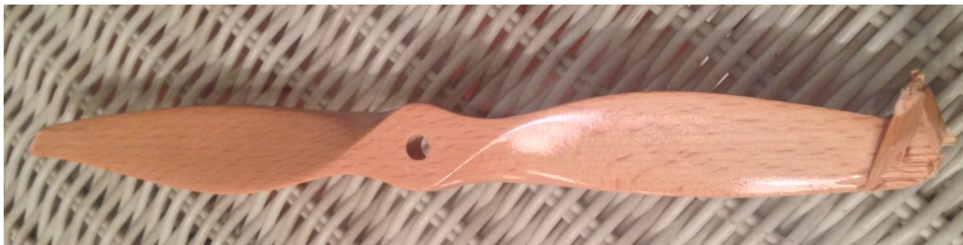
Figure 6.10: Broken propeller due to the crash.
