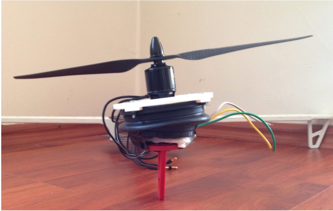
Figure 6.23: Tilt-roll rotor system for one motor is mounted on the body frame.
