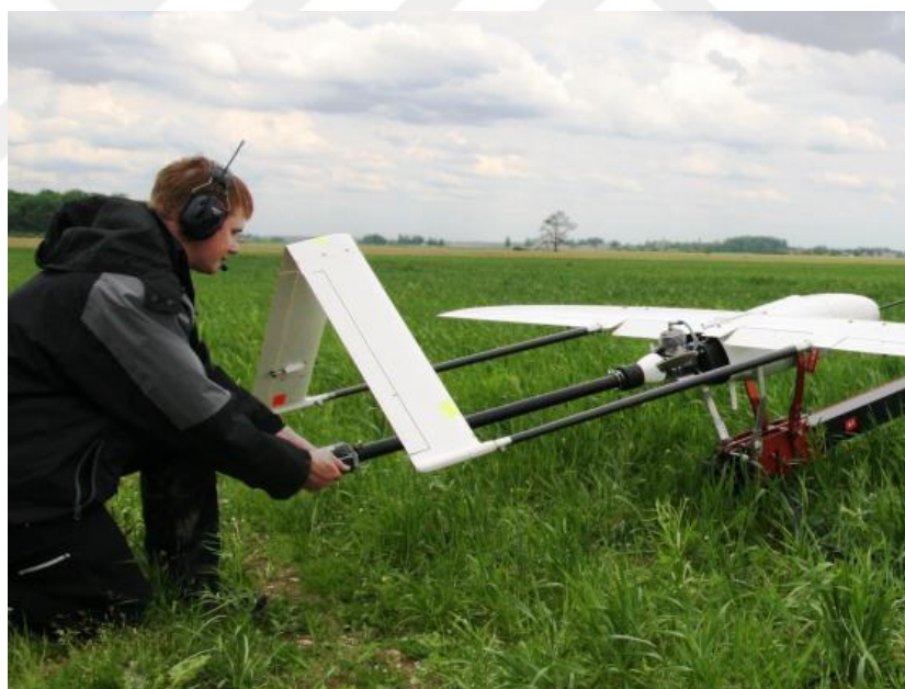
Figure 1.4 A Mini UAV Started With Engine Starter [13]
