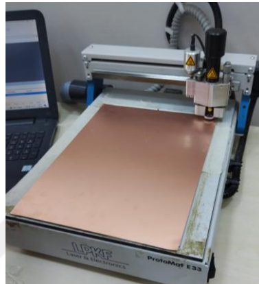
Figure 4.24 First step in the fabrication process, showing the laminated sheet positioned on the LPKF ProtoMat E33 milling machine.
