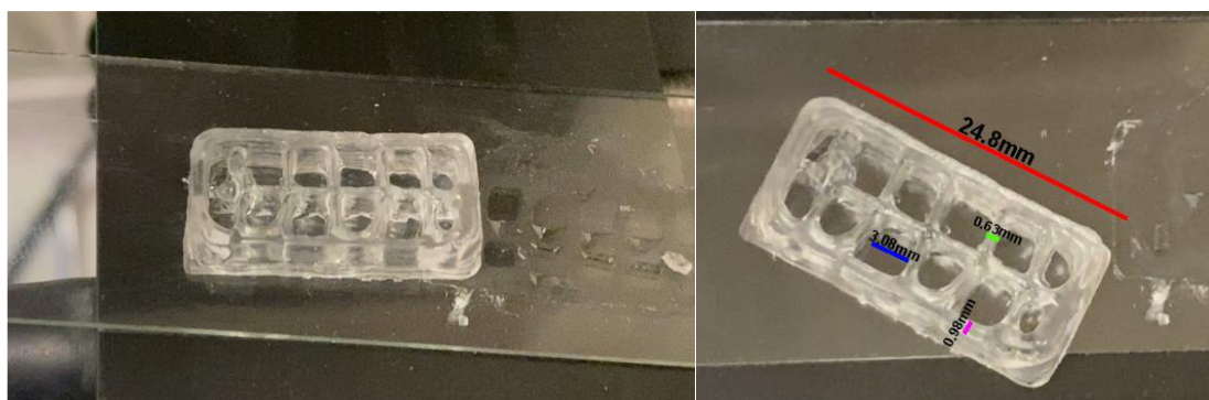
Fig. 17. Gelled grid structure after printing.
