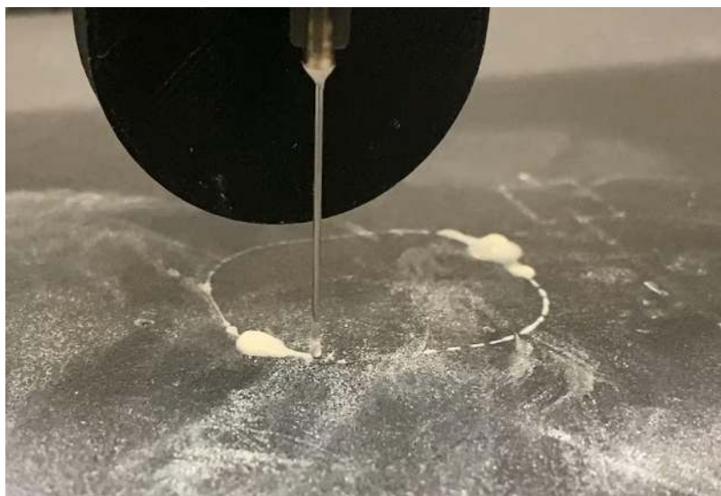
Fig 10. \text{TiO}_2 added ink with air bubbles during printing.
