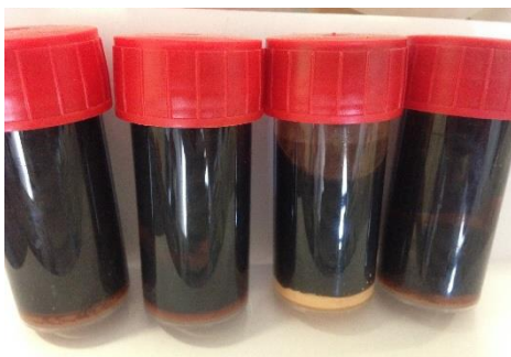
Figure 4-8: Gels with precipitated zirconium pigment with varying weight percentages
