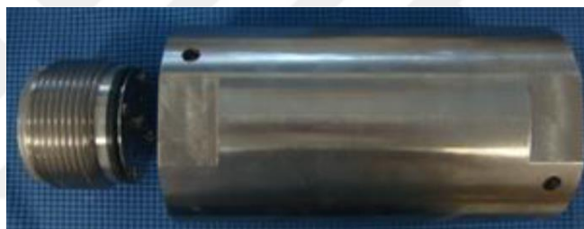
Figure 3-2: 500 mL vessel used for supercritical drying
