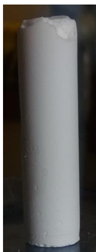
Figure 6.3. A photograph of the synthesized monolithic silica-titania aerogel composite with 50 wt% of titania.
