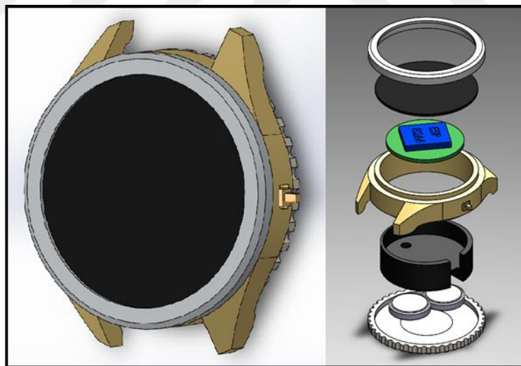
Figure 29 EHU's Template's Detailed Outlook (From Below to Above: Lower Case, 2 Batteries, Battery And Circuit Sockets (intermodulation), Main Component, Circuit (EHU), Glass and Upper Case)
