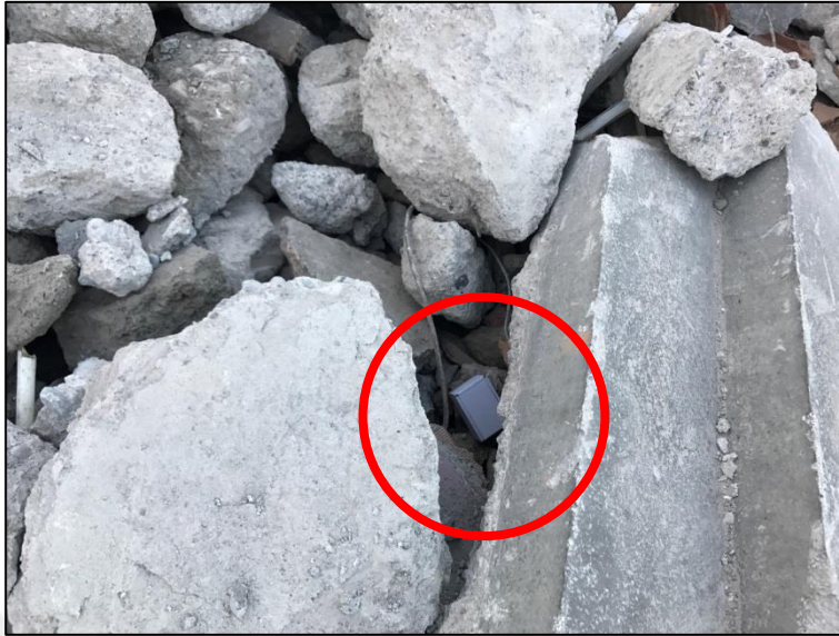
Figure 40 Placement of EHU In The Wreckage (Device II)
