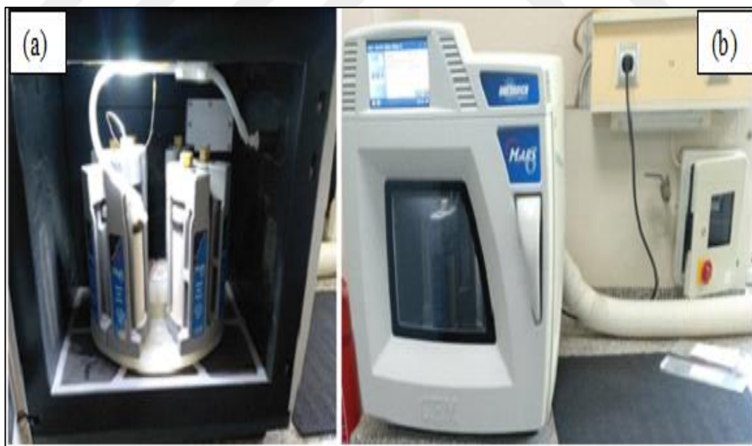
Figure 5.5 Image of CEM Microwave digestion system. (a) Vessels loading, (b) At the starting of microwave operation (Personal annal, 2021)
