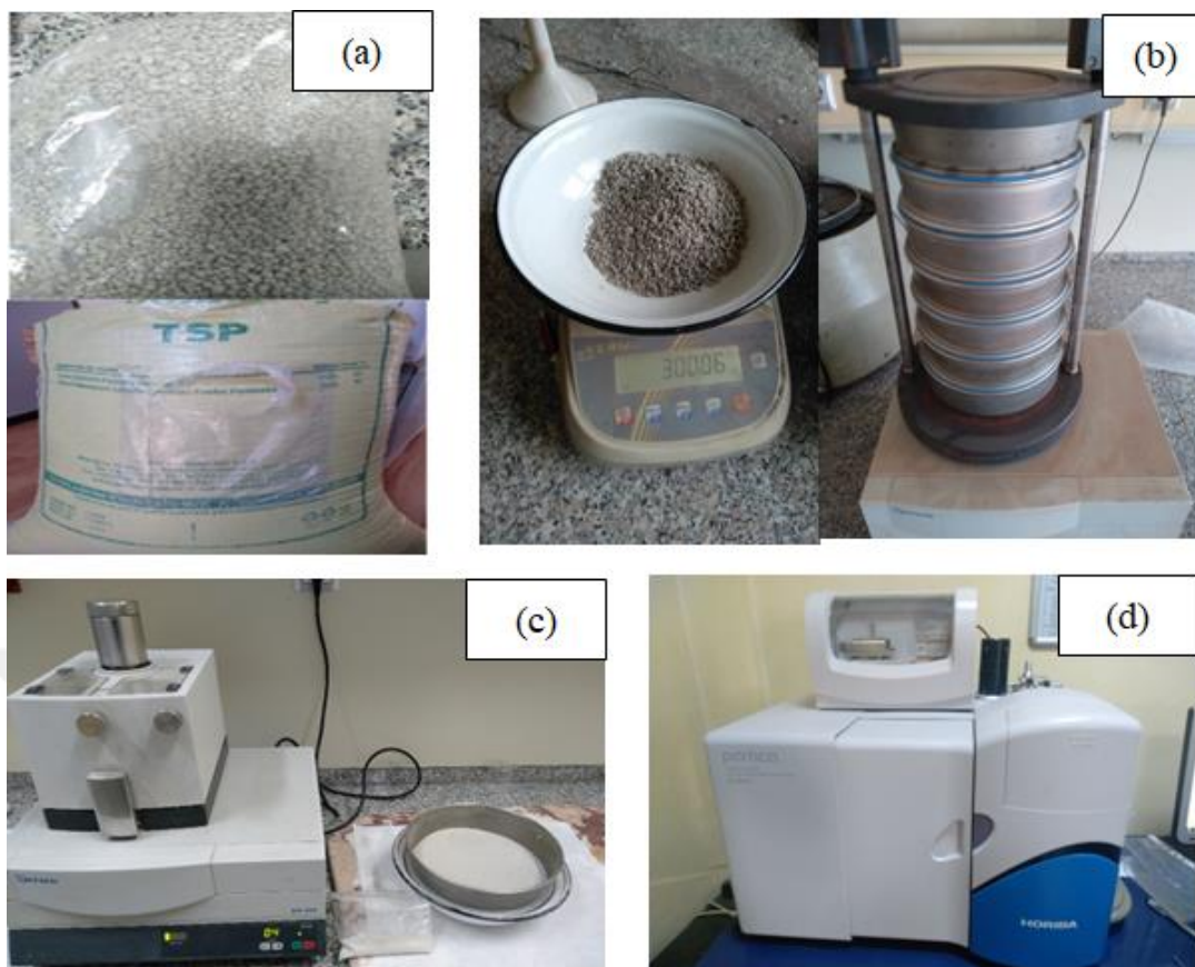
Figure 4.2 Grinding and particle size analyses of TSP. (a) TSP as received, (b) Particle size distribution analysis of granular TSP by vibratory sieving machine, (c) Grinding the granular TSP to size below 100µm MG100/MG200 mortar grinder, (d) Particle size analysis of ground TSP by Horiba LA-950 laser scattering device (Personal annal, 2019)
