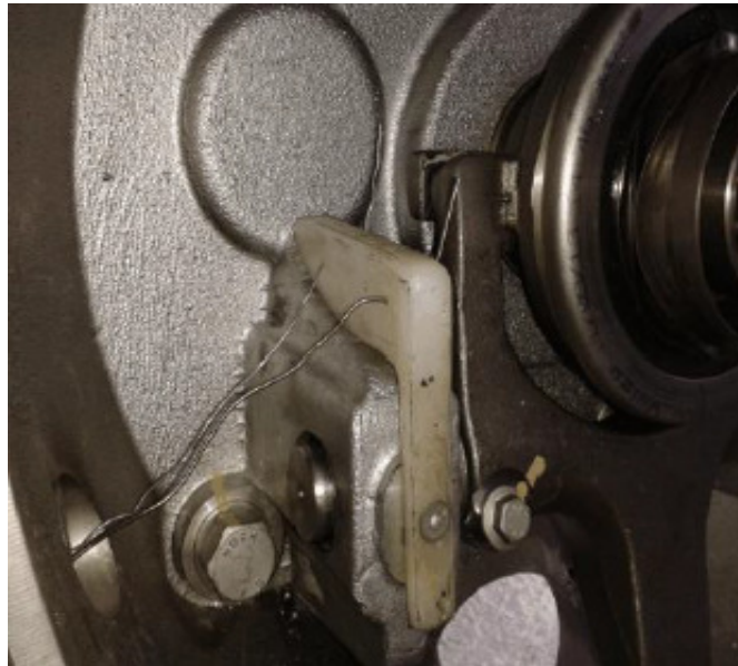
Figure 4.8 : Thermocouple position near clutch release bearing.
