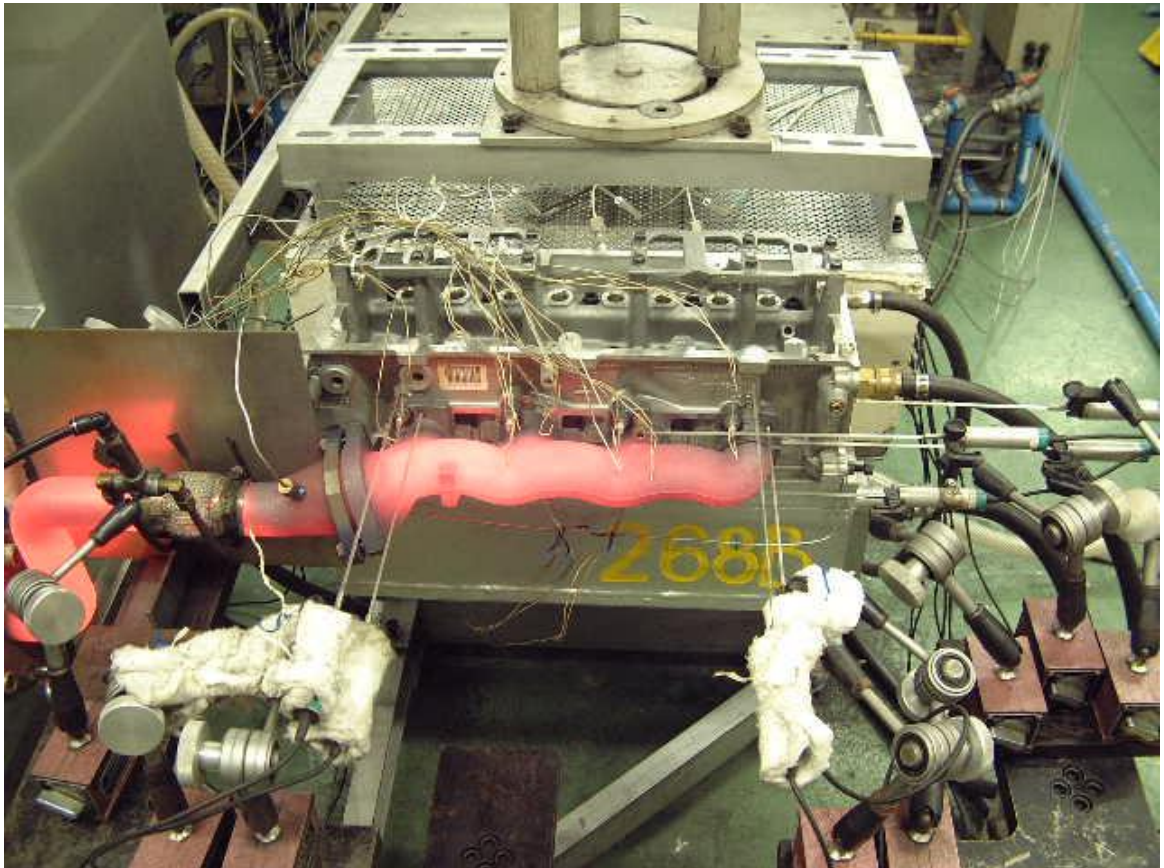
Figure 4.1: Experimental set-up at Hitachi-Japan showing the extensometer and thermocouple locations for an exhaust manifold.
