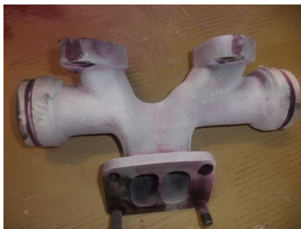
Figure 10.3 : Exhaust manifold center part after penetration.
