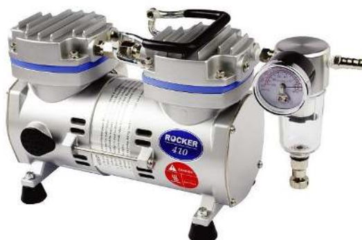
Figure 3.8 Vacuum Pump and Vapor sampling system
