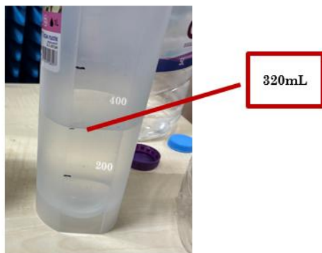
Figure 3.29. Calibration Flask to increase 2mm of height in Tank
