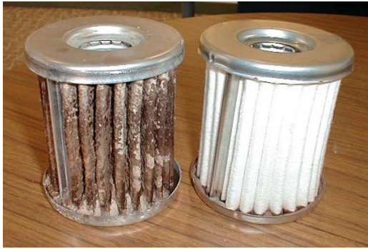
Figure 1.3. Effect of water contamination on motor spare parts
