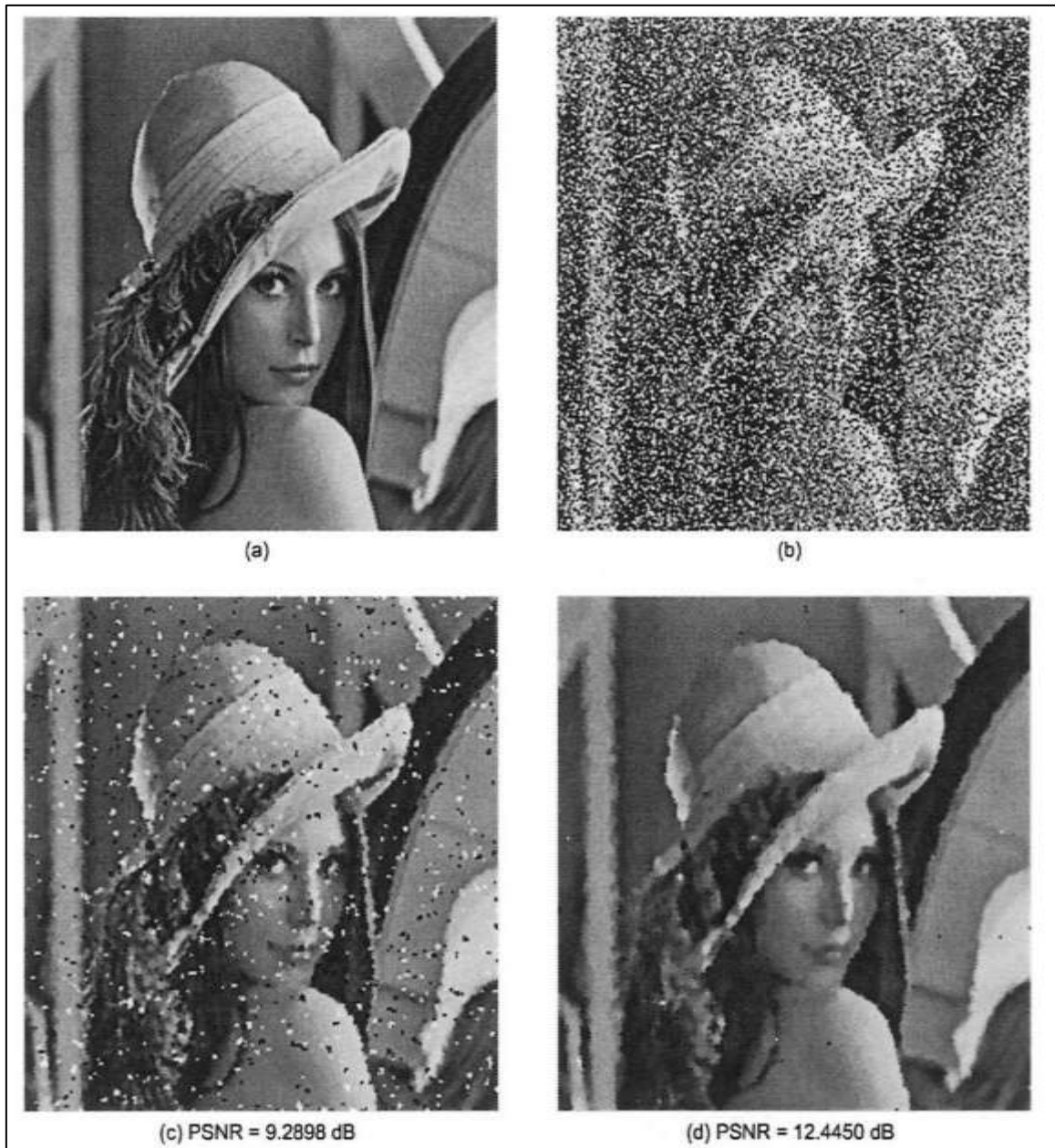
Figure 3.6: The Application of Nonlinear Filtering [5].
