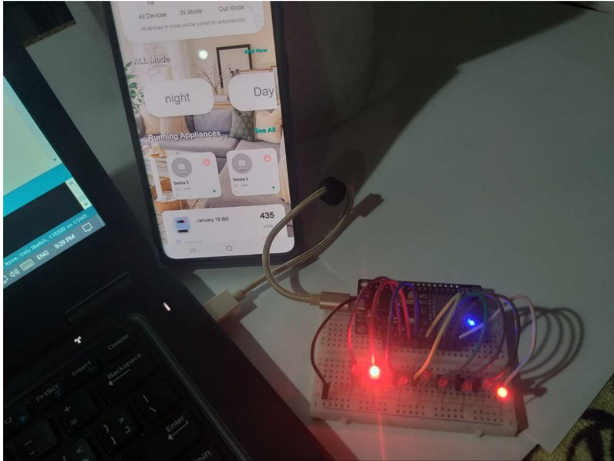
Figure 4.2: Image of the proposed smart meter
