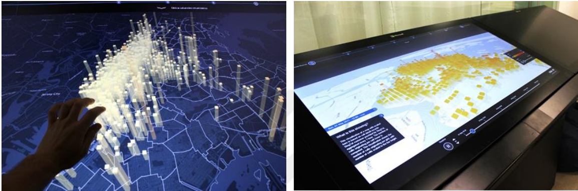
Figure 2-4 Data Drive, an interactive visualization tool for urban designers that allows to visualize and configure series of data set according to the inputs like transportation routes, parking locations, building energy consumption, etc. https://morphocode.com/v
