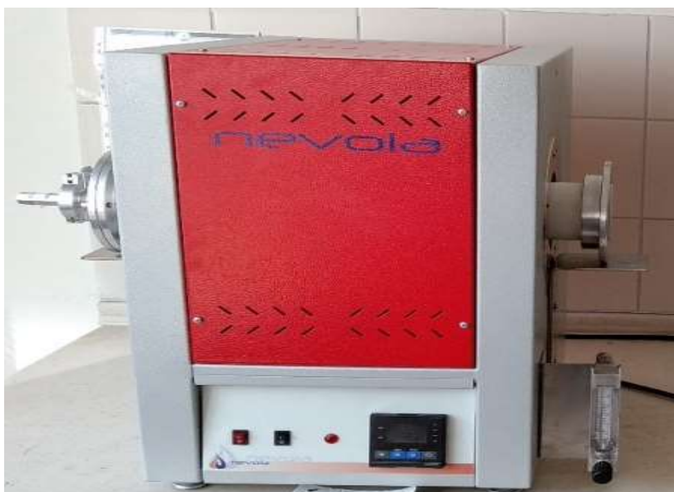
Figure 4.4. The electric tube furnace used for sintering
