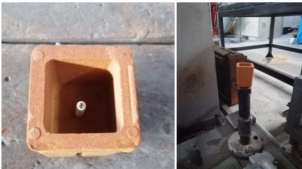
Figure 3.13 Thermocouple location in the Quick cap
