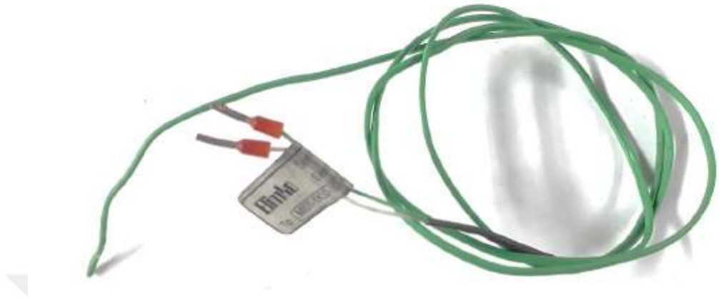
Figure 3.9 K type cable thermocouple [10]
