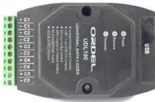
Figure 3.11 Ordel data logger temperature scanner connected to the computer [10]
