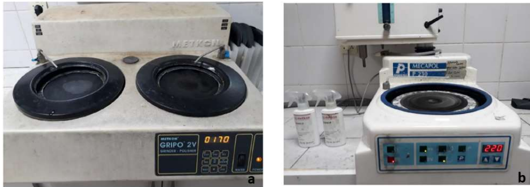
Figure 3.19 Rotating disc type a: Grinder, b: Polisher with 6 \mu and 1 \mu diamond solutions [10]
