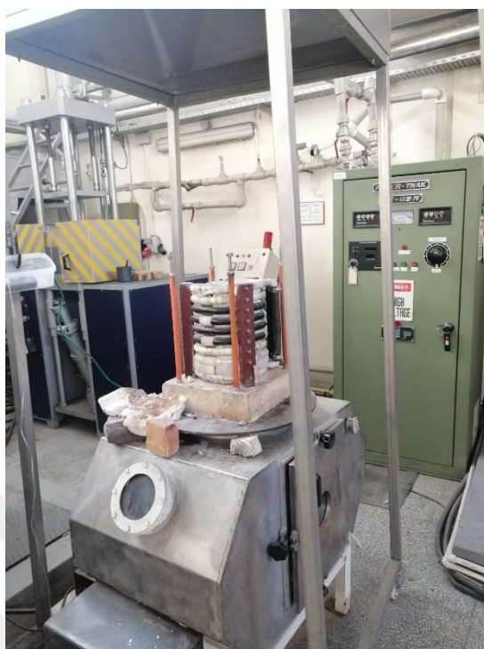
Figure 3.5 Induction Furnace “Prothoterm”
