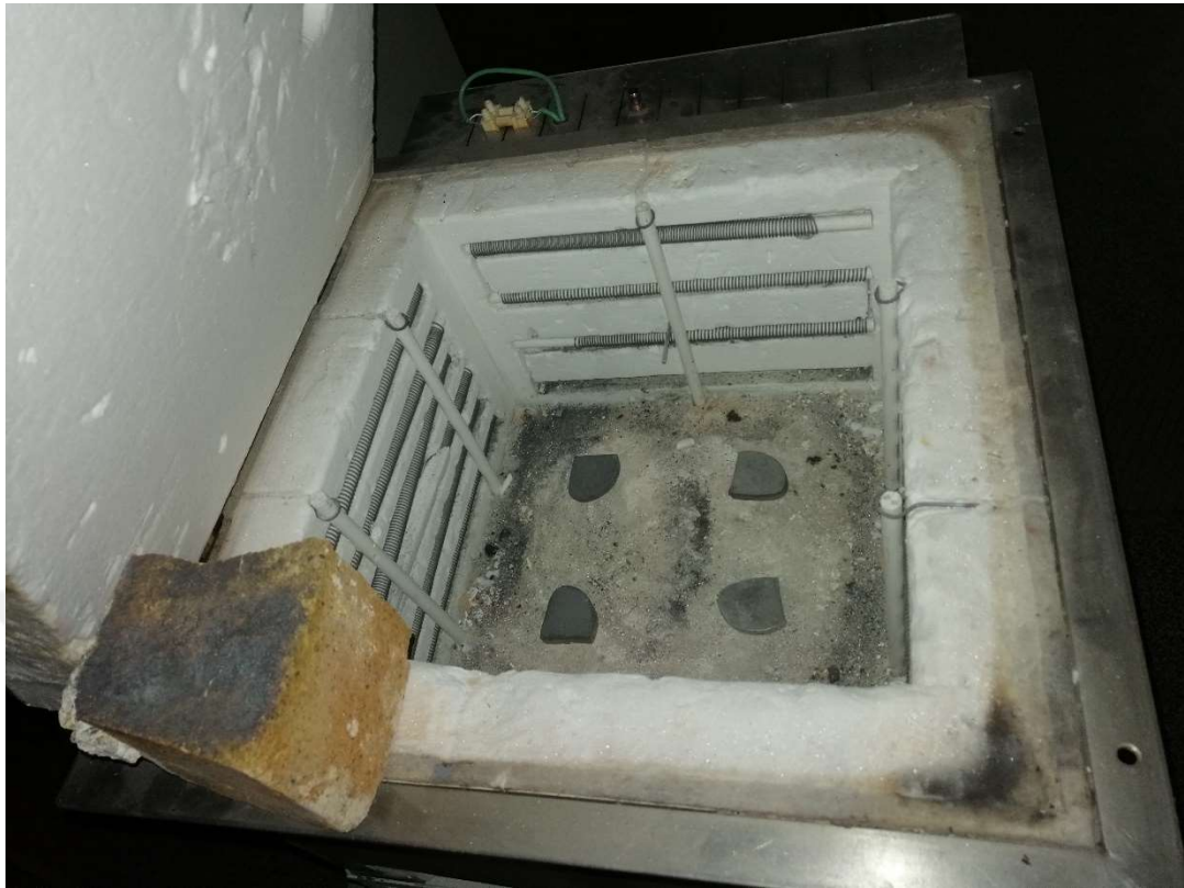
Figure 3.22 Electrical resistance furnace used for heat treatments
