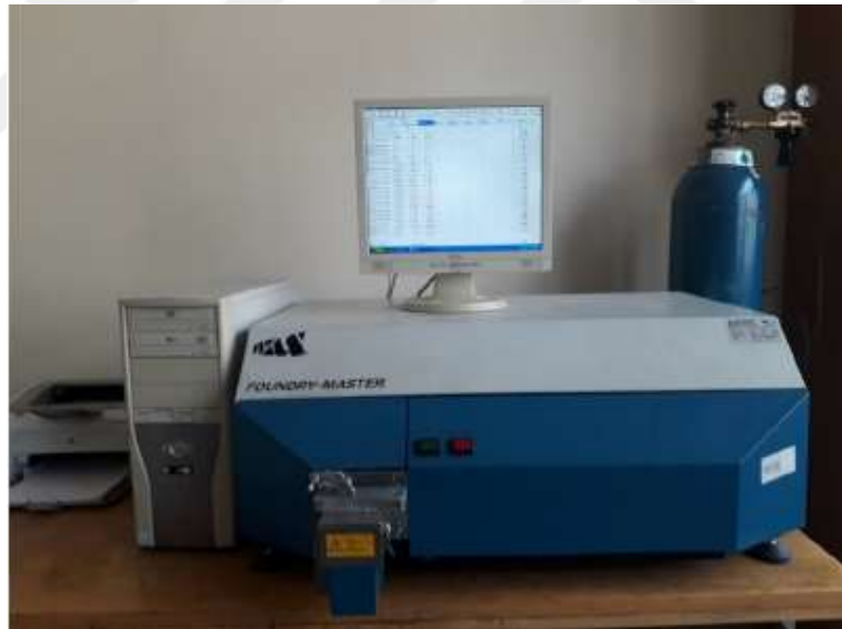
Figure 3.7 WAS Foundry Master optical emission spectroscopy [10]
