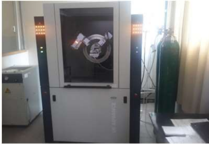
Figure 3.15 XRD instrument used for crystal structure analysis [10]
