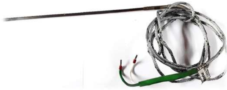
Figure 3.10 K type metal thermocouple [10]
