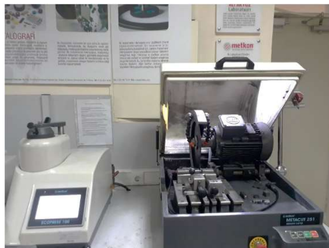
Figure 3.18 METACUT 251 grinding cutter (right) and the mounting bakelite device (left) [10]
