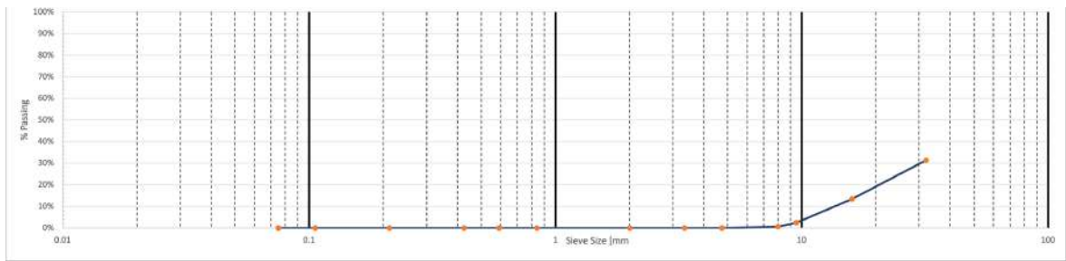
Figure D. 60. Sediment grading graph for K26 -2m sample.
