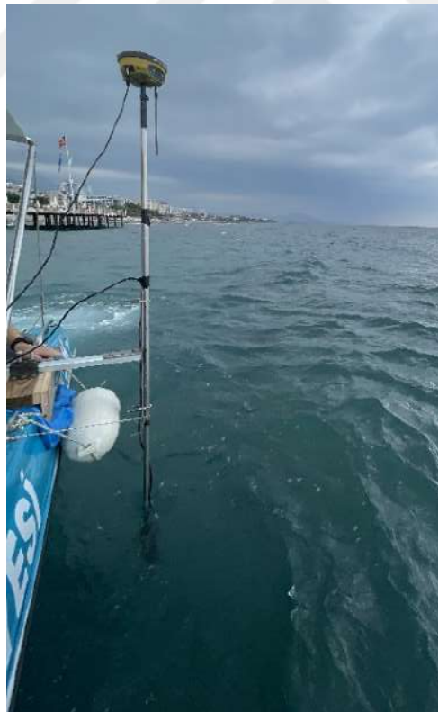
Figure 3.6. Single beam echo sounder device attached to GPS rover.
