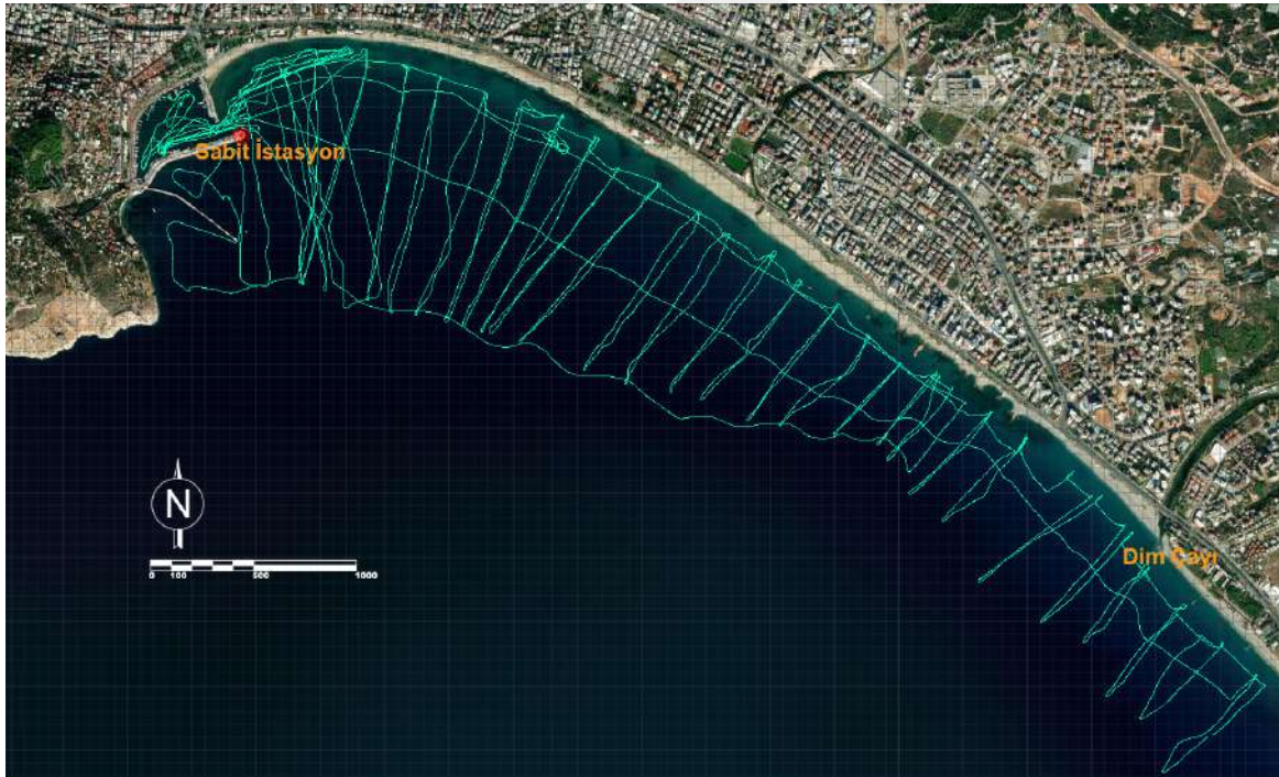
Figure 4.1. Boat survey trajectory.
