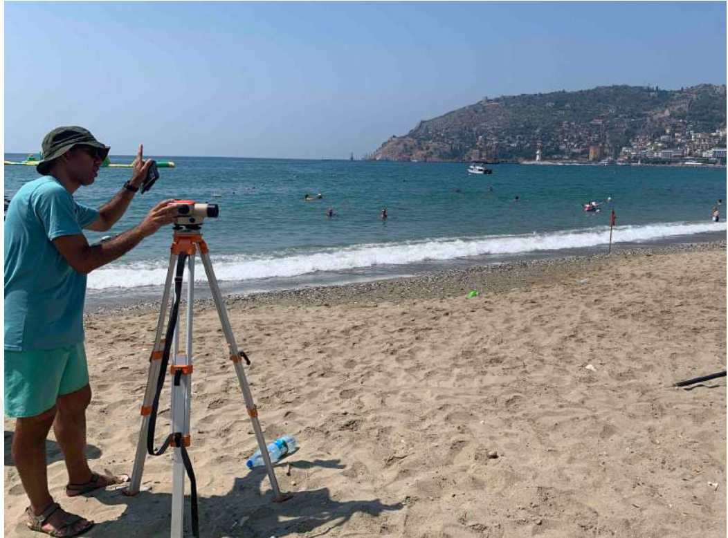
Figure 3.2. Measurement of wading profiles with leveling device.
