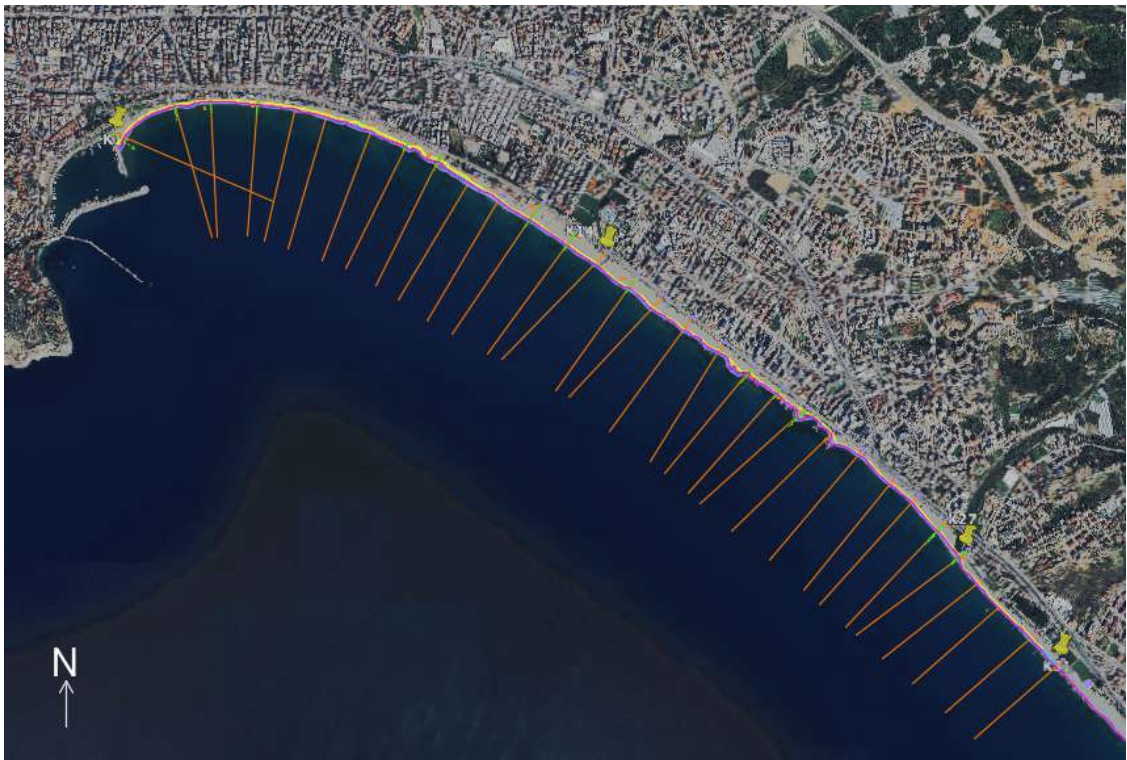
Figure 3.3. Profile sections and survey area shown on map.
