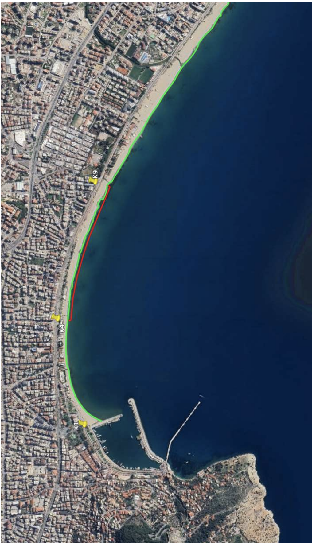
Figure 4.24. Nourishment design between section K4 and K9 shown on map.
