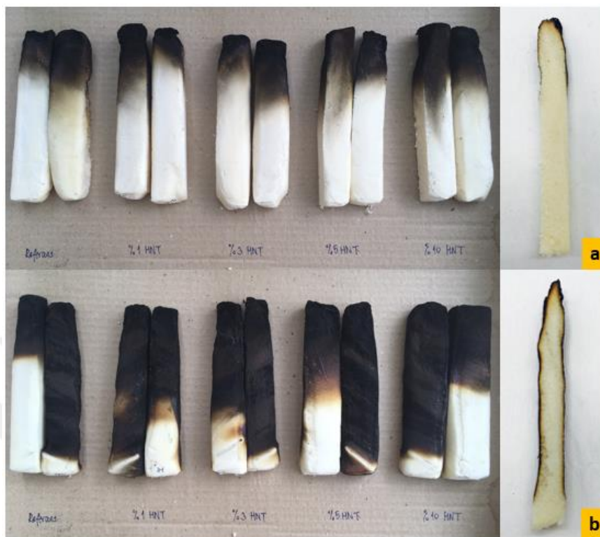
Figure 39. Tested (a) SP (b) DEC foam samples and on the right-side of the images, cross sections of the reference samples
