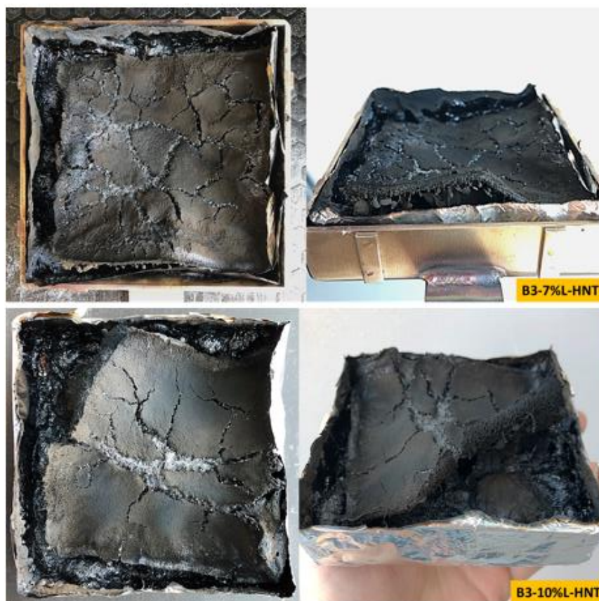
Figure 44. Appearance of the samples incorporated with L-HNT after testing with cone calorimeter
