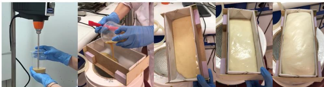
Figure 7. Sample preparation for small flame test
