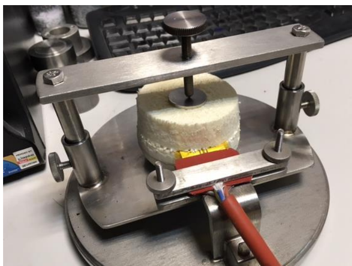
Figure 6. Thermal conductivity measurement setup
