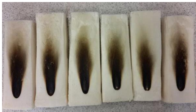
Figure 38. 1% HNT loaded SP foam samples after testing with small flame test
