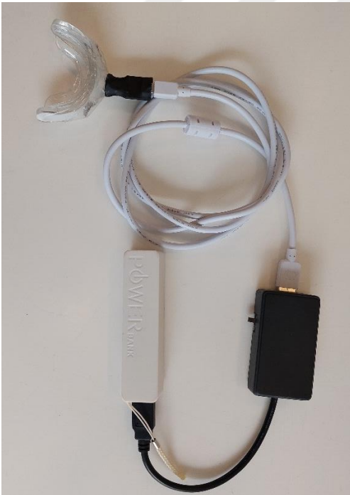
Figure. 3.5. A sample of the device prepared to be delivered to patients. Working with usb and powerbank.
