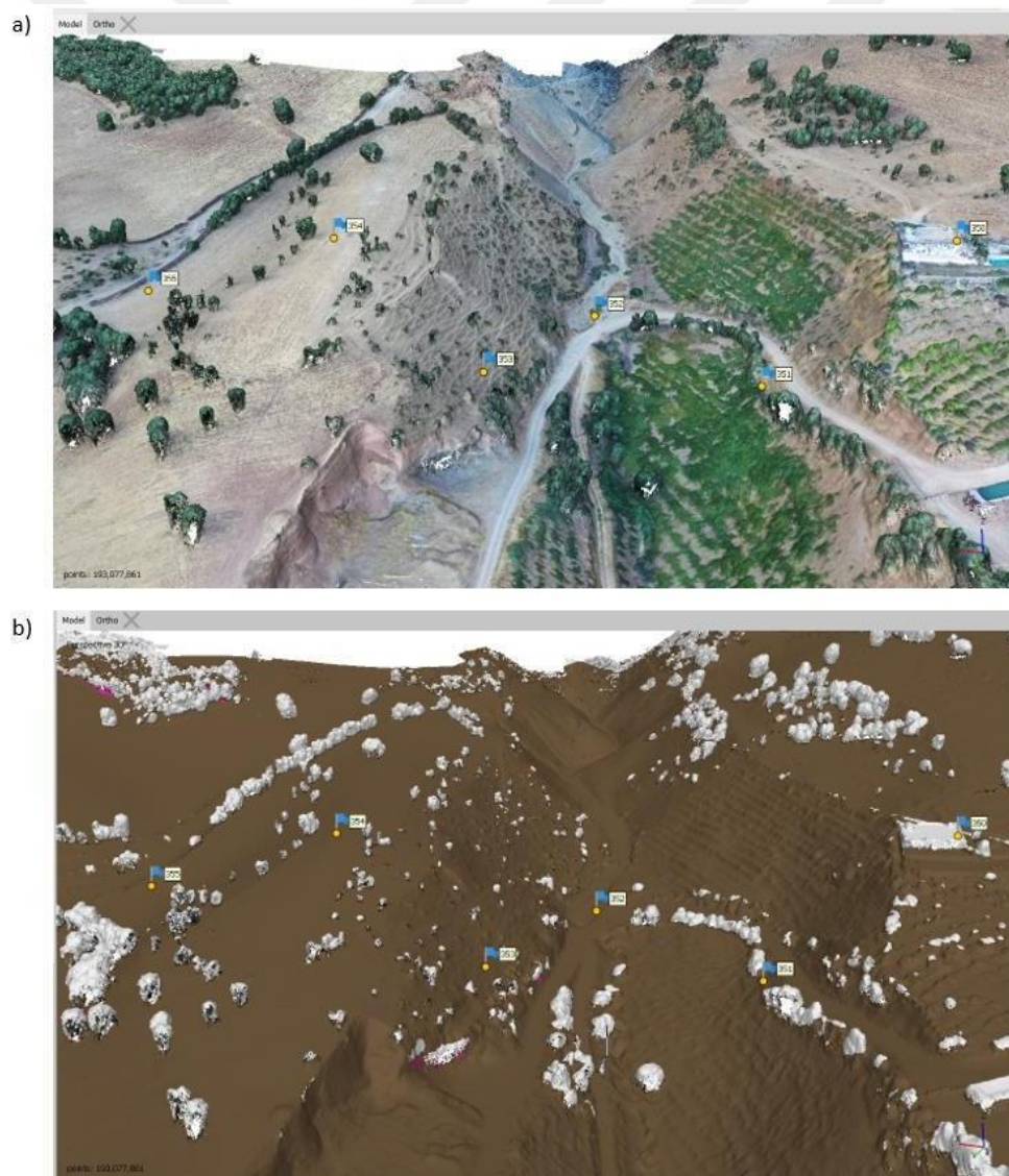
Figure 27. Generating all Points Clouds (a). Generating Ground Points Clouds (b)
