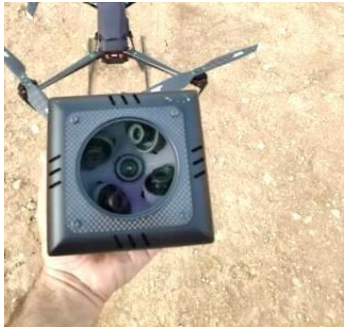
Figure 18. Foxtech 3DM V4 oblique camera
