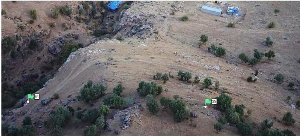
Figure 20. GCPs irregularly placed on the slope and flat surface.
