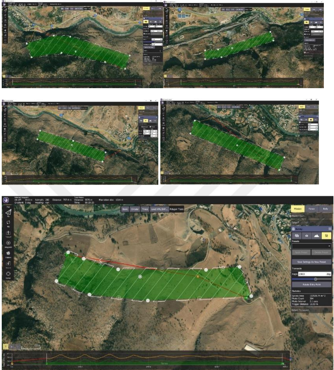
Figure 24. Flight mission plan by QGround Control software
