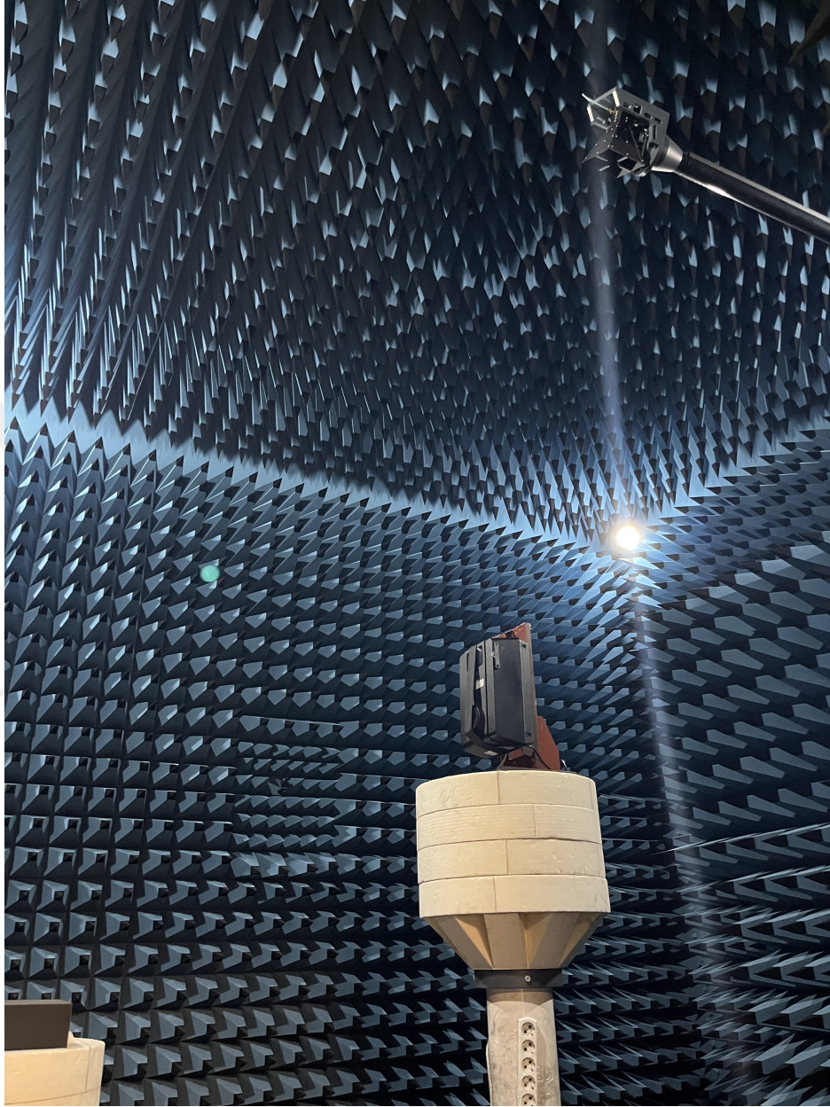
Figure 7.1: An anechoic chamber is a structure whose interior surfaces are covered with pyramidal RF absorbers that attenuate electromagnetic waves and block external EMI. This allows antenna radiation patterns, TRP, and TIS measurements to be performed without multipath effects.
