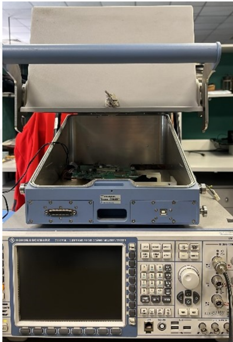
Figure 8.3: Baseboard placed inside a shielded box for conducted receiver sensitivity measurements.
