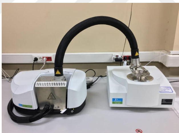
Figure 3.5. Thermogravimetric analyser coupled with a Fourier-transform infrared spectrometer present at the Composite Material Characterisation Laboratory, Center for Wind and Energy Research, Middle East Technical University.
