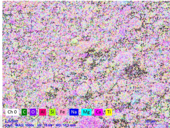
Figure 30. EDS elemental analysis (mapping) of virgin L Schist including Si, Al, Ca, Mg, Fe, Na, Ti, C, and O
