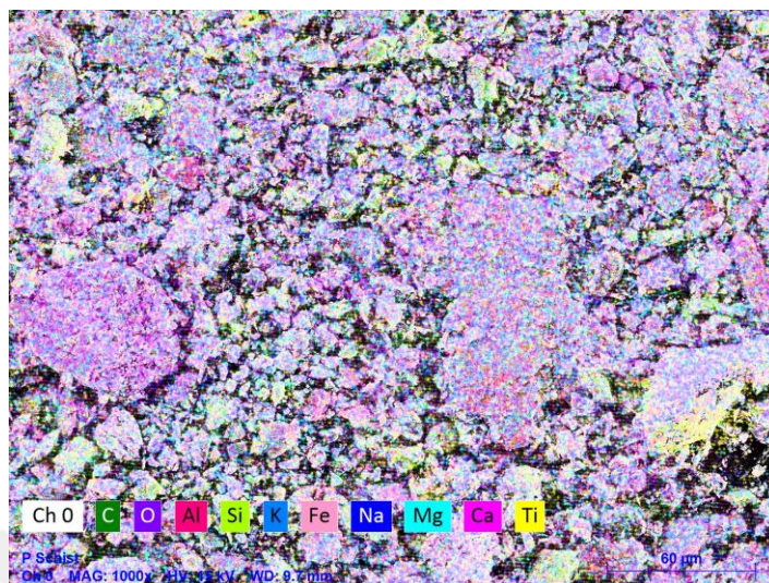
Figure 28. EDS elemental analysis (mapping) of virgin P Schist including Si, Al, Ca, K, Mg, Fe, Na, Ti, C, and O
