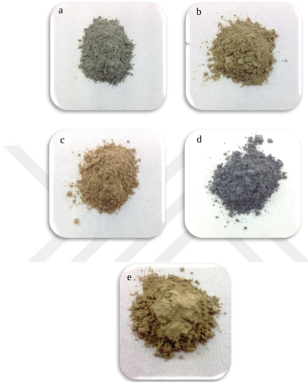
Figure 8. Ground powder schist-type samples ready for activation as a) G, b) C, c) P, d) B, and e) L
