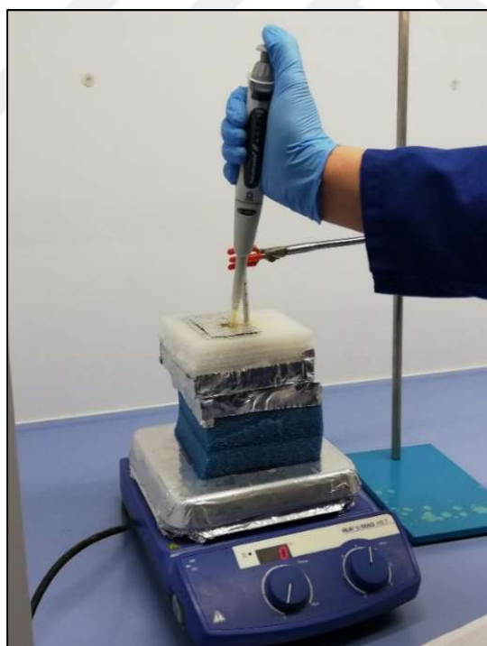
Figure 3.2. Injection of oxidizer into coffee-cup calorimeter
