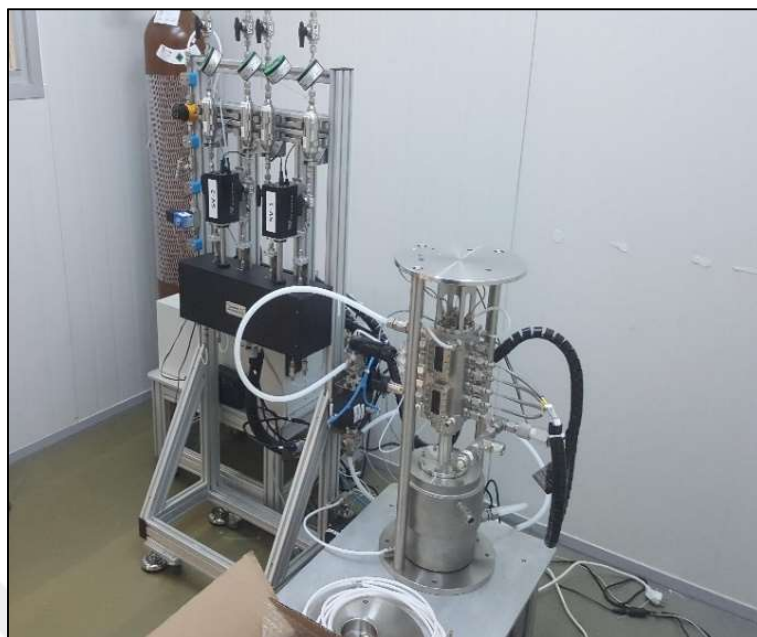
Figure 7.1 The Impinging jets reactor experimental setup
