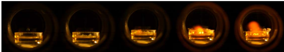
Figure 3.6. The instants of dropping, collision, ignition and combustion in IDT
