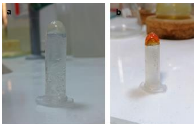
Figure 1.37. Gel formations of (a) P16 (b) P18 by using co-solvent system.
