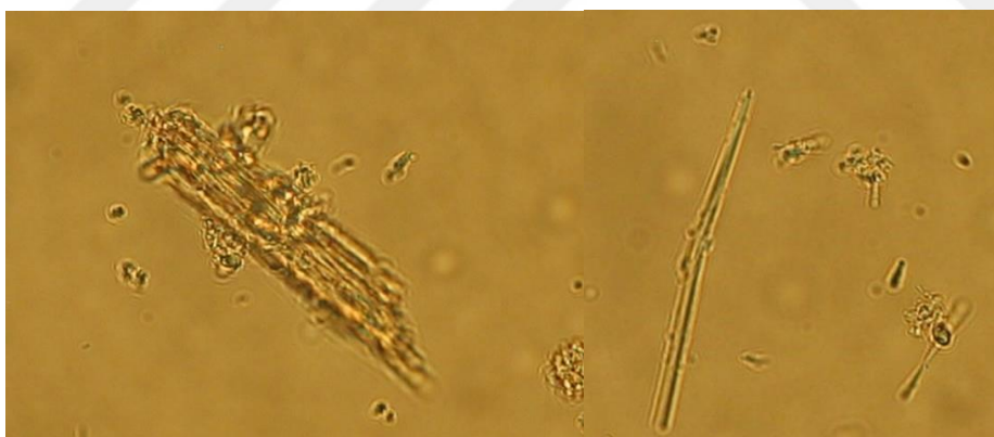
Figure 1.34. Microscope image of microcrystals of P8 obtained after self-assembly.
