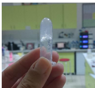
Figure 1.35. The gelation of mixed P12-P13 after pH adjustment.
