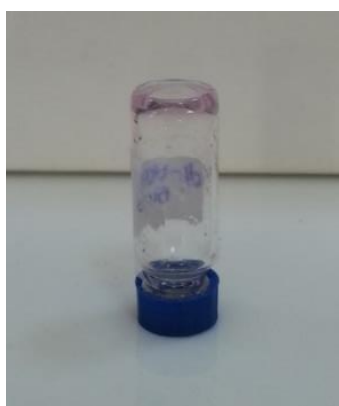
Figure 1.33. P3 gel in pH 7.5 Tris.HCl buffer. The sample did not flow by inversion of the vial.
