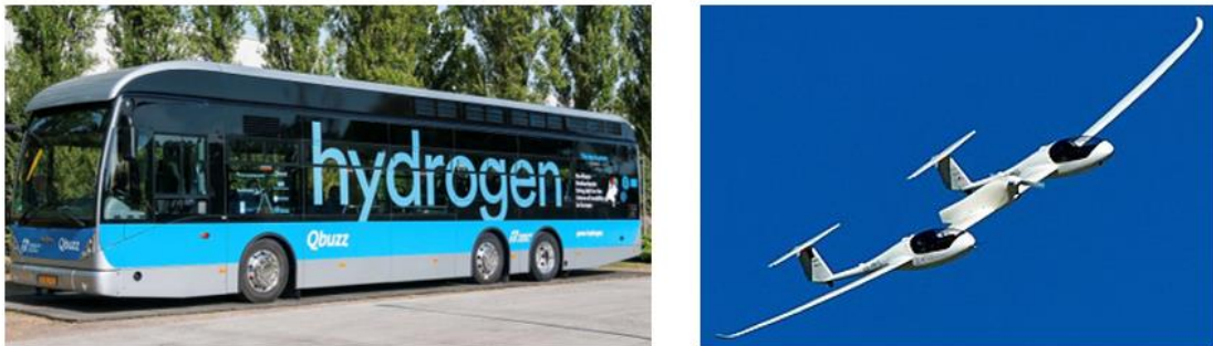
Figure 1.1: Hydrogen powered bus (Ballard Power Systems, Qbuzz) and passenger aircraft (HY4, DLR)
