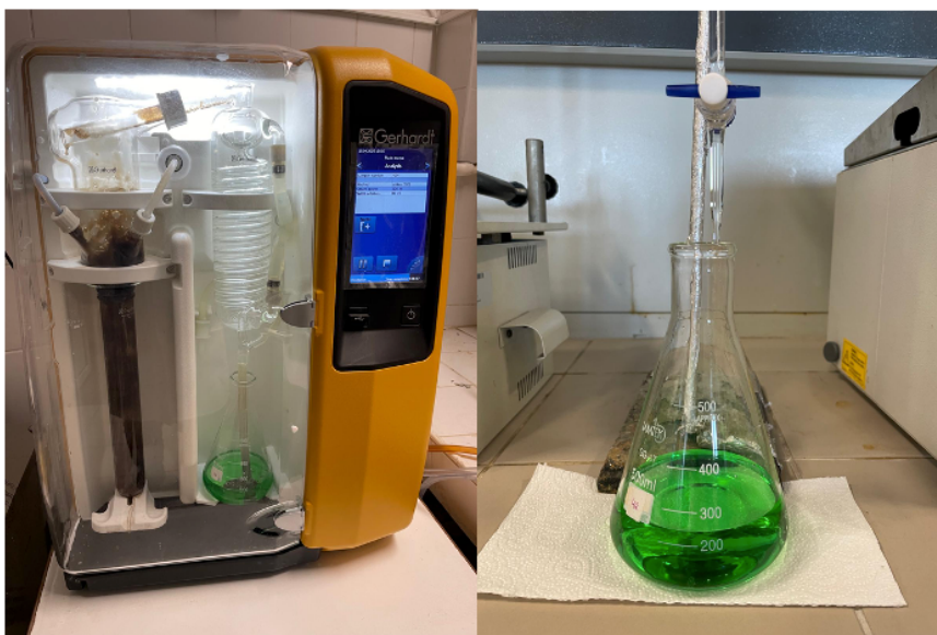
Figure 4.7. Gerhardt device for Kjeldahl nitrogen determination and titration unit.
