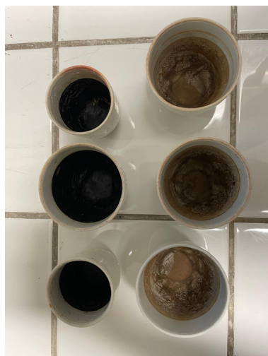
Figure 4.5. Crucibles used in TS and VS analyses.
