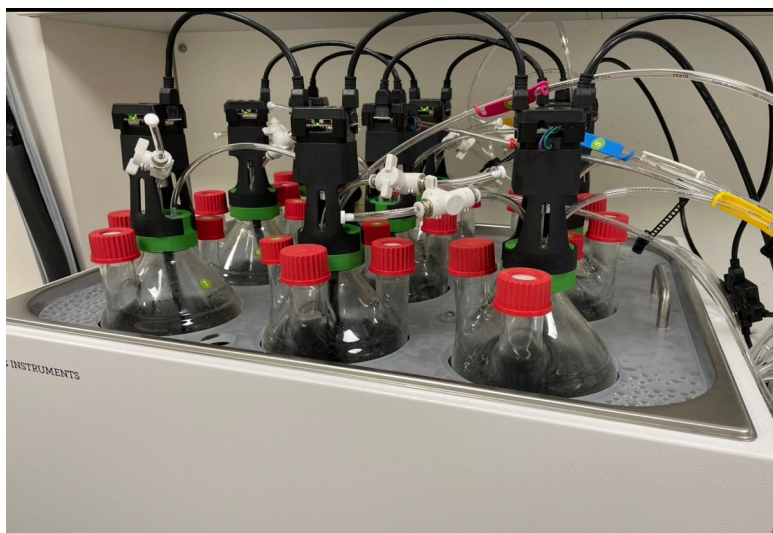
Figure 4.8. Water bath integrated experiment reactors.
