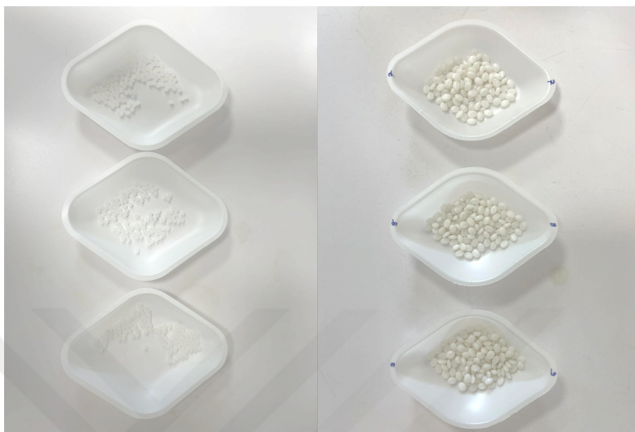
Figure 4.3. PLA pellets (on the left) and PBAT pellets (on the right).
